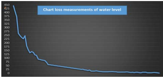
Figure 5. Grout curtain proof test for right hand sealing technic (water level decline from 2015/02/22 to 2015/05/21)
