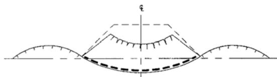
Figure 3. Settlement of soft subsoil under embankment loads (Holtz et al. 1998)
