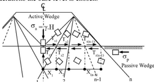
Figure 4. Fan of discontinuities for sliding forces and resisting forces due at a depth near to surface level
