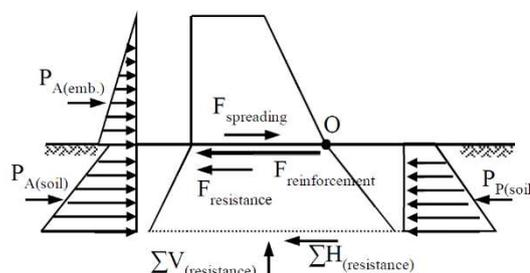
Figure 5. Reinforcement at the base level of embankment against lateral spreading effect
