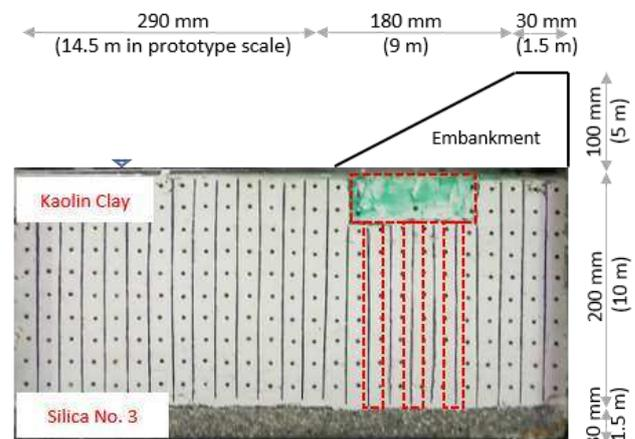
Figure 11: Model ground of centrifuge model tests (Nguyen et al. ICSMGE 2017)
