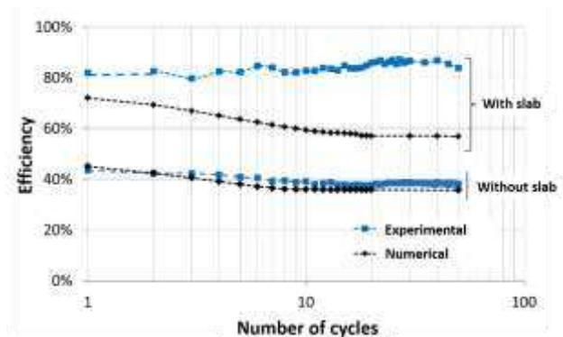
Figure 9: Evolution of the load efficiency with the number of cycles (Houda et al. ICSMGE 2017)
