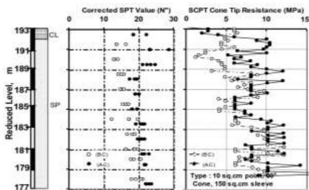
Figure 2. SPT and SCPT before (BC) and after compaction (AC) (Gupta et al. ICSMGE 2017)
