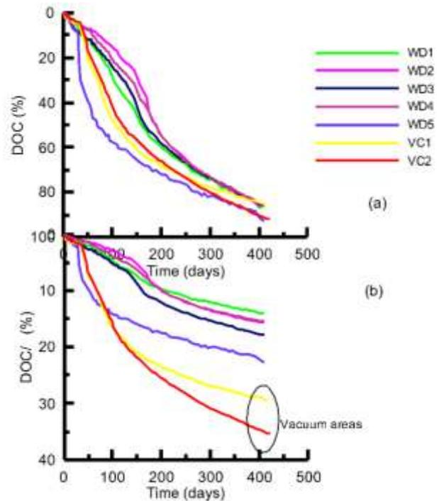
Figure 4. Degree of consolidation (a) before normalizing and (b) after normalizing (Rujikiatkamjorn and Indraratna ICSMGE 2017)
