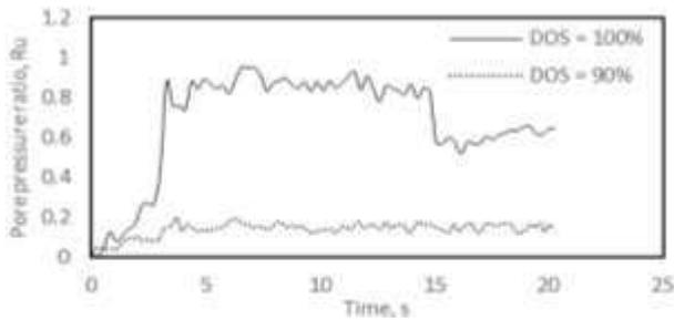
Figure 7: Change of pore water pressure during vibrations (Wu et al. ICSMGE 2017)
