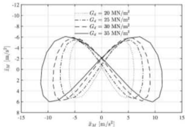
Figure 1. Theoretical shape of the accelerations during compaction (Pistor et al. ICSMGE 2017)
