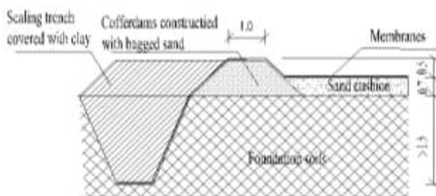
Figure 3. Relationship among the temporary cofferdams, sand cushion and sealing trench (Liu et al. ICSMGE 2017)
