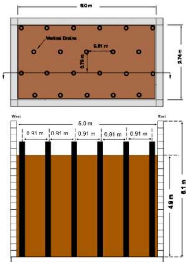
Figure 6. Plan and profile of laminar shear box with vertical drains (Rollins and Oakes ICSMGE 2017)
