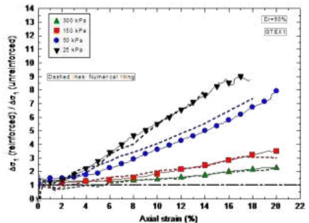
Figure 8: Ratio of axial stress increment (reinforced/unreinforced samples) (Miranda et al. ICSMGE 2017)
