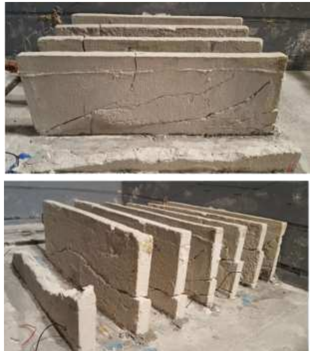
Figure 4. Photographs of the soil-cement walls during model excavation after testing; embankment toe was to the left side of both photos.
