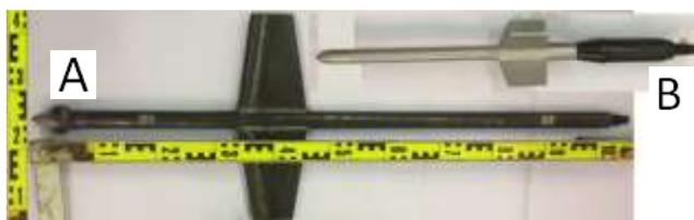
Figure 1. Column (A) and vane penetrometer (B) for columns. The dimensions of the tip A are presented in the standard EN14679 (2005) and in handbook (Forsman et al. 2015) and of tip B in handbook.
