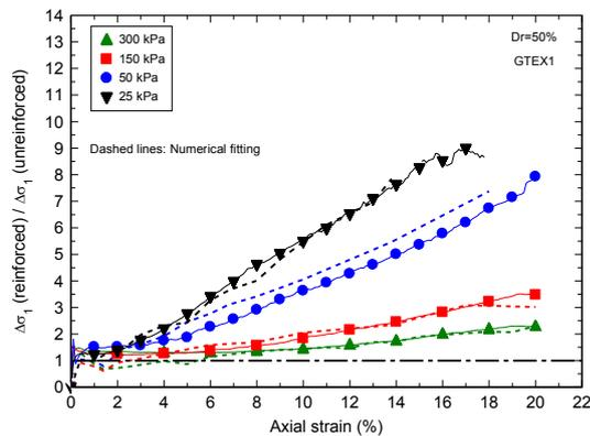
Figure 4. Numerical result for the ratio of axial stress increment (reinforced/unreinforced samples)
