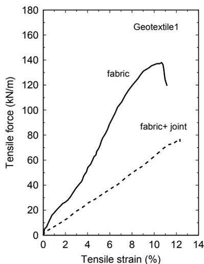
Figure 1. Tensile force versus strain of the geotextiles.
