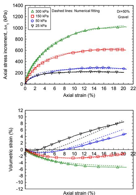
Figure 2. Numerical fitting of the drained triaxial tests of the gravel
