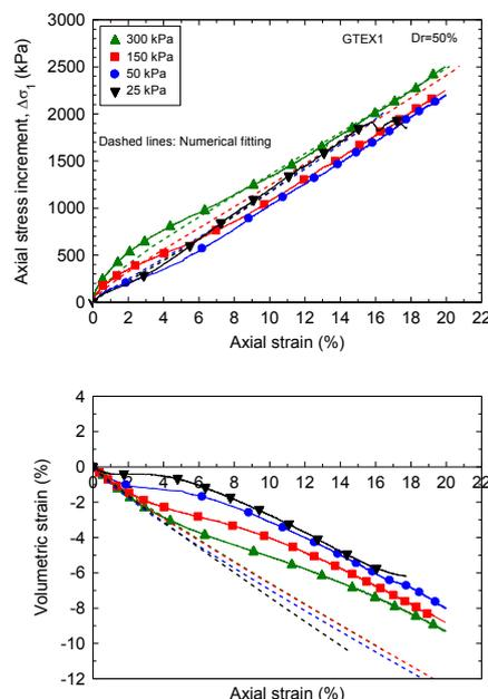
Figure 3. Numerical results of the drained triaxial tests in samples encased with geotextile1
