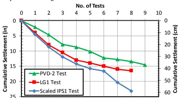
Figure 5. Cumulative settlement versus number of shaking tests in laminar box with drains (PVD-2 Test) in comparison with laminar box without drains (LG-1 and IPS1 Test).
