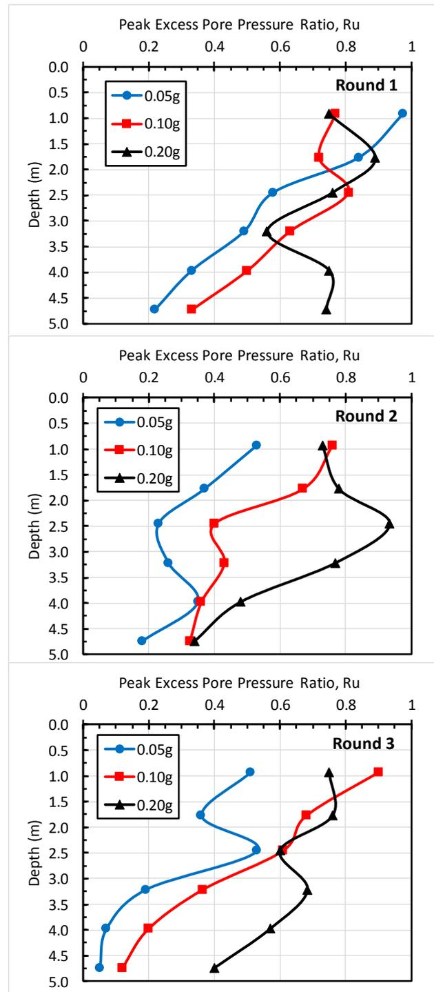
Figure 4 Peak excess pore pressure ratio for three arrays vs. depth plots for round 1, 2, and 3 test with 0.05, 0.10, and 0.20g base input motions per round. Peak values are averages at each depth for three transducers.
