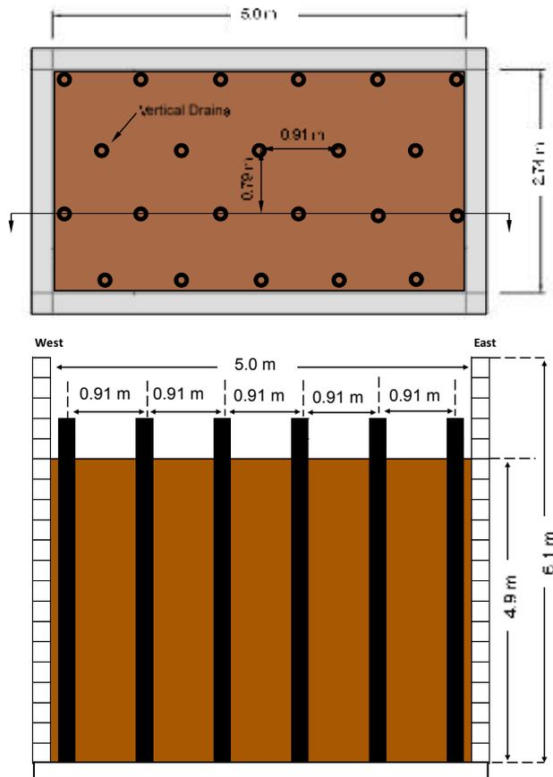
Figure 1. Plan and profile views of the laminar shear box with vertical drains in triangular pattern spaced at 0.9 m on centers.
