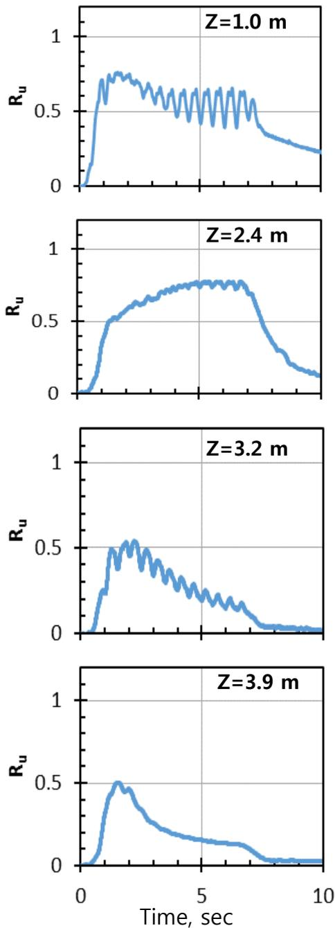
Figure 3 Excess pore pressure ratio time histories measured by pore pressure transducers located at 1.0, 2.4, 3.2, and 3.9 m below the ground surface for the 0.1g peak acceleration motion during round 1 testing.
