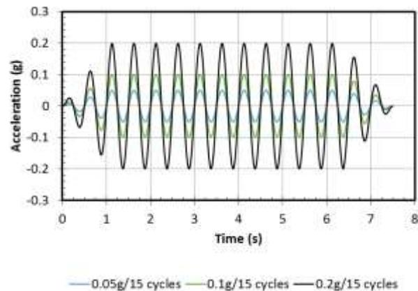
Figure 2. Base input motions for each round of shaking.
