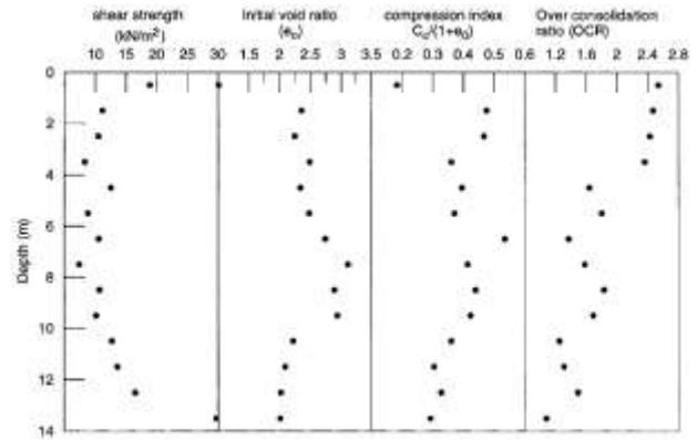
Figure 4. Basic properties of soft clayey deposits at SBIA (Indraratna et al. 2005c).
