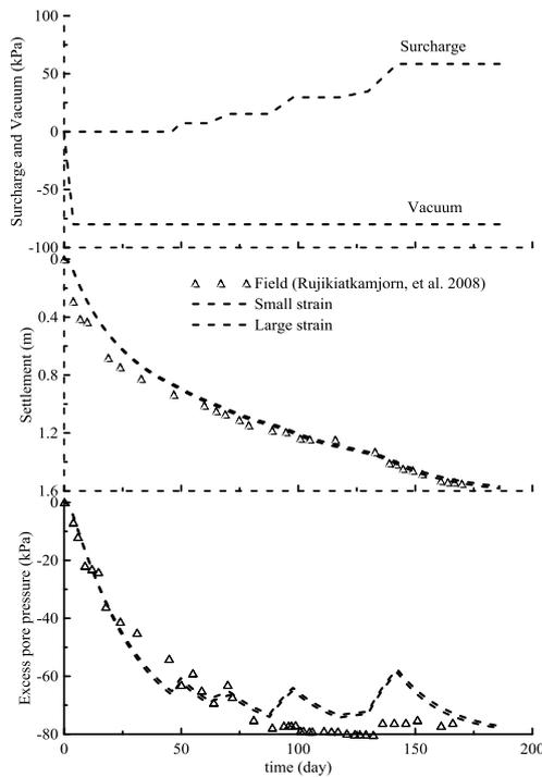
Figure 3. Load history, settlement and excess pore pressure at the project at Tianjin Port
