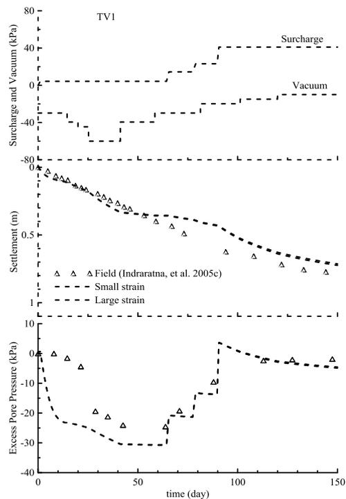
Figure 5. Prediction and field measurement of settlement and excess pore pressure (3 m depth) at TV1 of SBIA.
