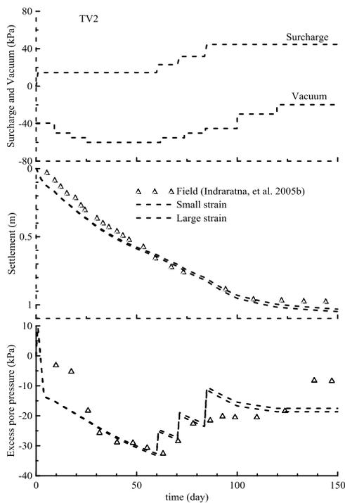
Figure 6 Prediction and field measurement of settlement and excess pore pressure (3 m depth) at TV2 of SBIA.
