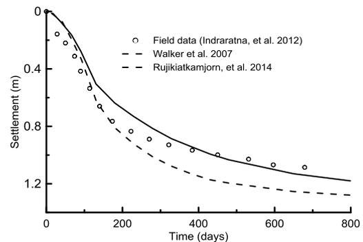
Figure 2. Predicted and measured settlement at SP1 of Ballina bypass (after Rujikiatkamjorn, et al. 2014).
