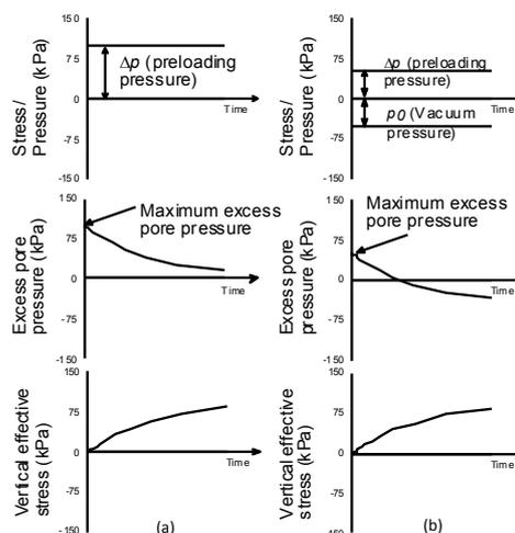
Figure 1. Principle of surcharge and vacuum preloadings (Indraratna et al. 2005c).
