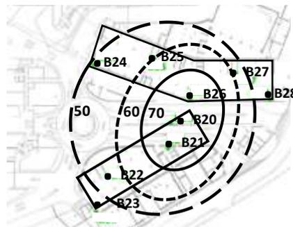
Figure 6. Measured settlement trough (mm) by structural load (after raft construction). Values to be multiplied by 1,4 to extrapolate to settlement at final load.
