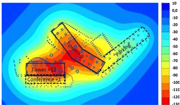
Figure 4. Calculated surface settlements (mm) at final load (maximum value 124,7 mm); the 9 and 12 level towers, adjacent low rise buildings and pile locations (dots) are indicated.
