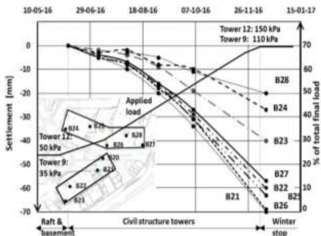
Figure 5. Settlement curves (after raft) as function of applied loading. At the winterstop, 70% of the final load applies to the foundation as finishing and shell are not yet constructed.
