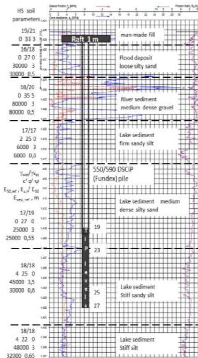
Figure 1. Lithological description, typical CPT and Hardening Soil parameters used for FEM
