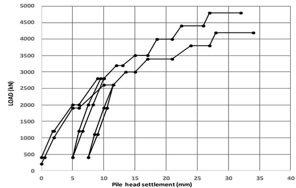
Figure 3. Static load test.  $\varnothing 590/550$ mm DSCiP (Fundex) pile length 26 m and 27 m.
