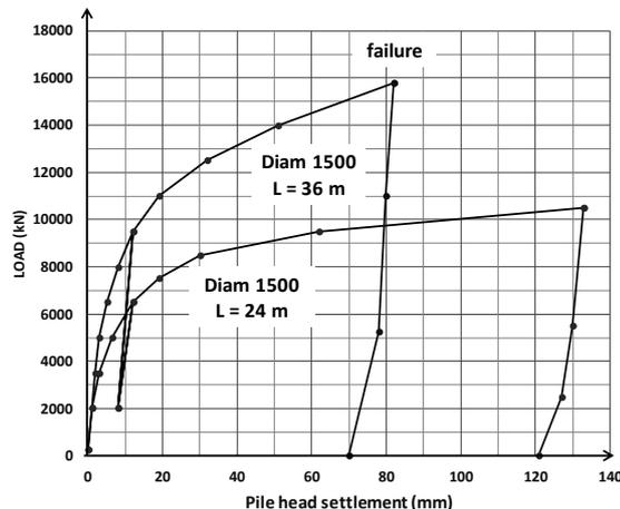
Figure 2. Static load test.  $\varnothing 1500$ mm Bored piles 24 m and 36 m
