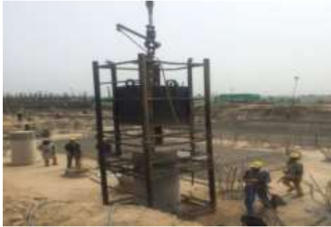
Fig. 5: Setup for Dynamic Load Test (DLT)
