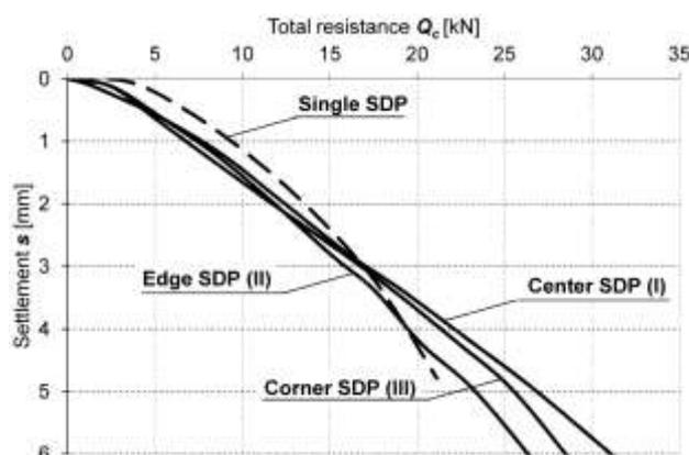
Figure 11.  $Q$ - $s$  graphs of model scale SDP piles working individually and in a group.
