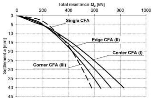
Figure 9.  $Q$ - $s$  characteristics comparison of CFA piles working in a group and as an individual pile.
