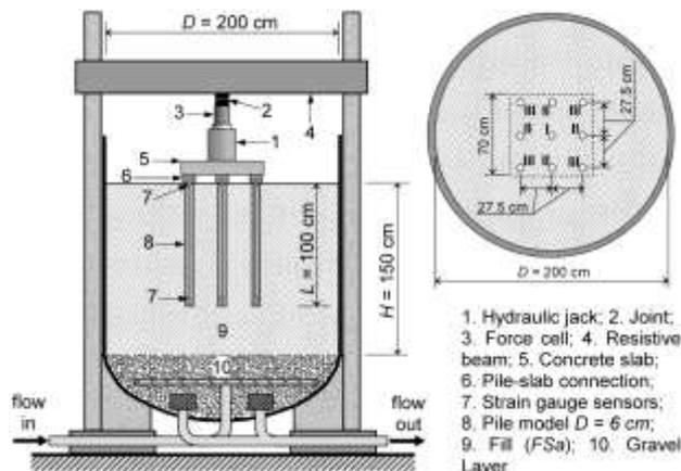
Figure 10. Model test site with pile arrangement plane.
