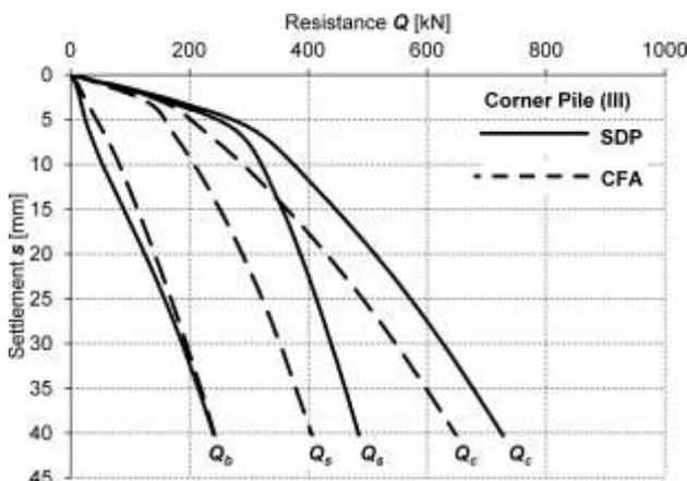
Figure 7. Calculation results presented as  $Q$ - $s$  curves for corner pile in group.
