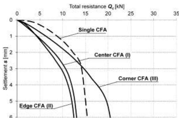
Figure 12.  $Q$ - $s$  graphs of model scale CFA piles working individually and in a group.
