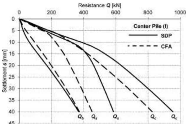
Figure 5. Calculation results presented as  $Q$ - $s$  curves for center pile in group.
