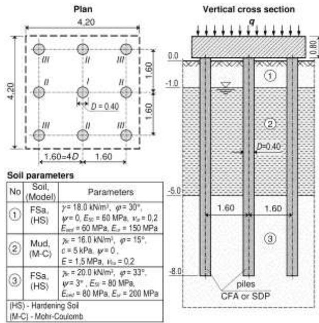
Figure 1. Material and geometrical data of pile foundation for FEM analyses.
