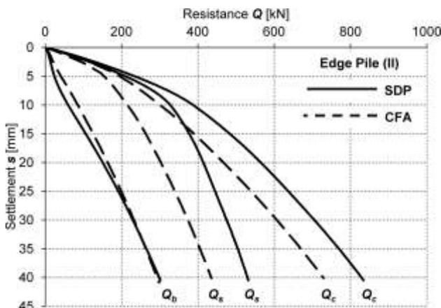
Figure 6. Calculation results presented as  $Q$ - $s$  curves for edge pile in group.
