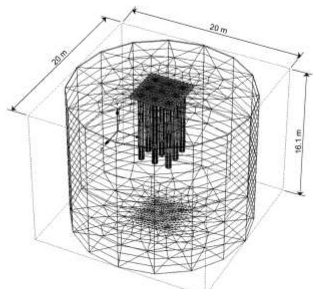
Figure 4. Calculation scheme for piles group FEM computation.
