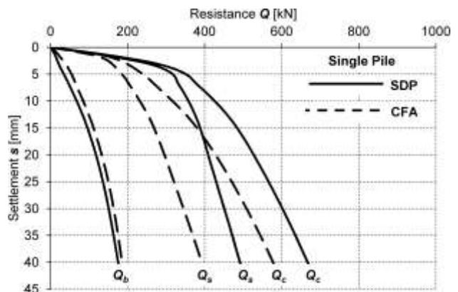
Figure 3. Calculation results presented as  $Q-s$  curves for single SDP and CFA piles.
