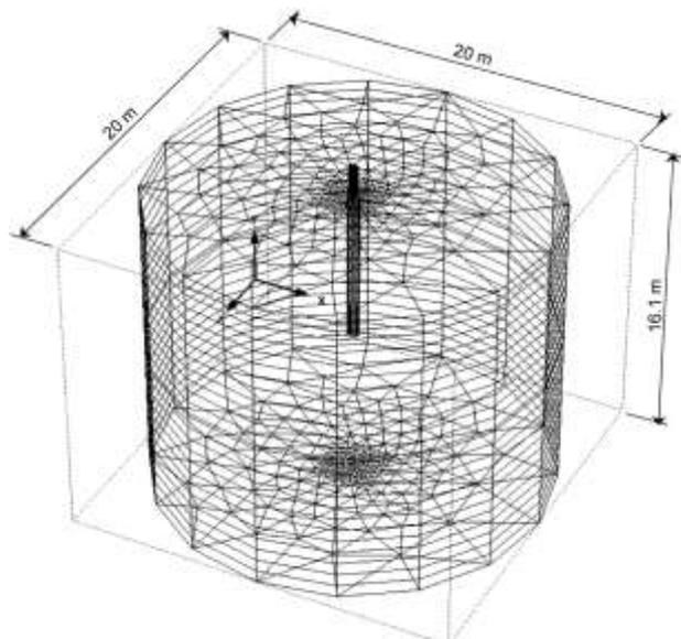
Figure 2. Calculation scheme for single pile FEM computation.
