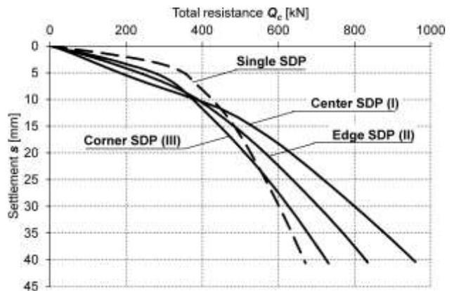
Figure 8.  $Q$ - $s$  characteristics comparison of SDP piles working in a group and as an individual pile.
