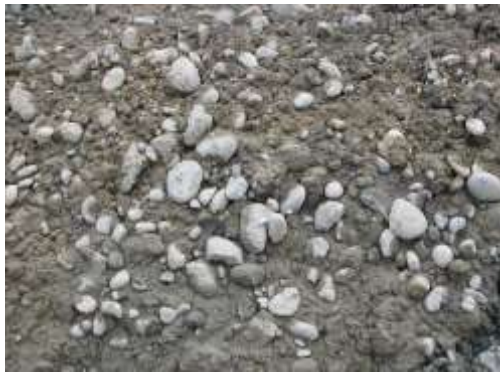
Figure 1. The properties of gravel and in-filled soil in open voids between weathered cobble-size andesite rocks.
