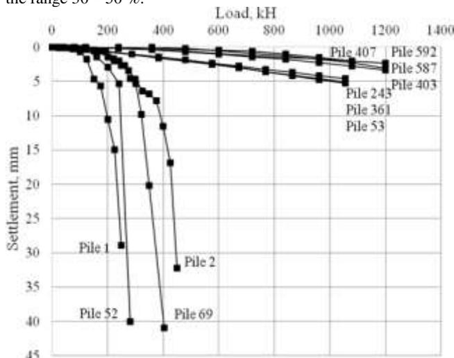
Figure 2. The pile settlement on soft clays (Pile №№ 1, 2, 52, 69), stiff clays (Pile №№ 53, 243, 361) and claystones (Pile №№ 403, 407, 587, 592).
