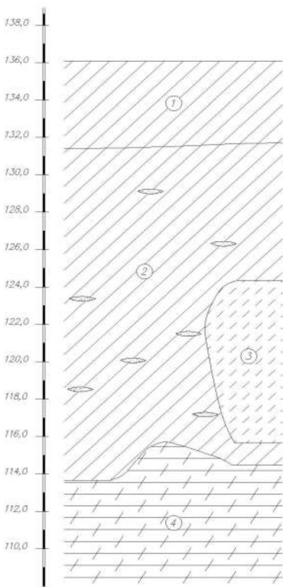
Figure 1. Experimental sites typical soil profile. Herein: 1 – soft loam and clay, 2 - soft clay and loam, with areas of gravel, 3 - loamy sand; 4 – claystone
