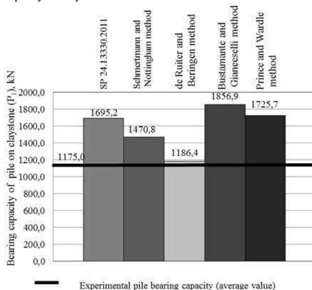
Figure 4. The average values of pile bearing capacity on claystones
