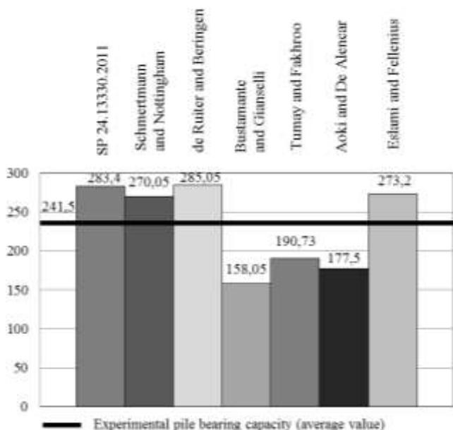
Figure 3. The average values of pile bearing capacity on soft clays
