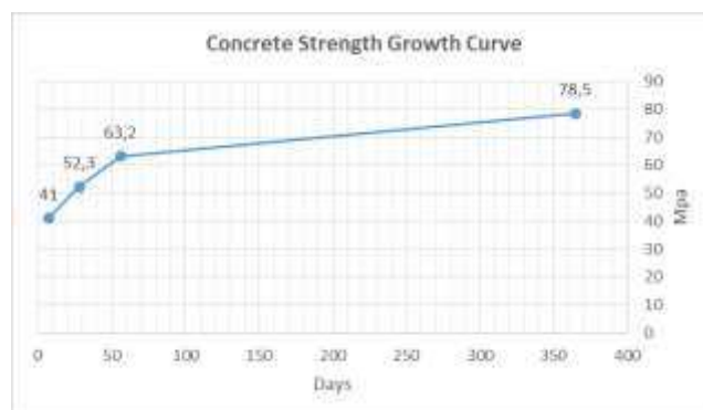
Figure 5. Concrete strength development until 365 days
