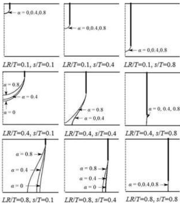
Figure 2. Behavior of the equipotential lines with cofferdam geometry.
