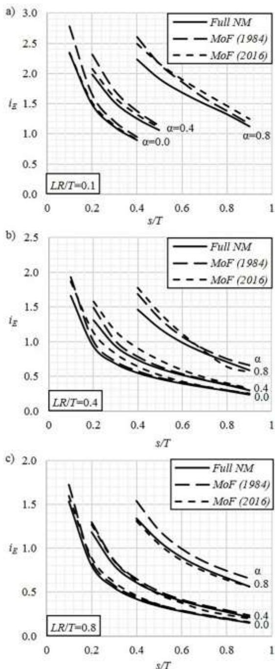
Figure 4. Comparison of the exit gradient.
