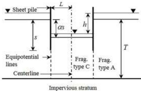
Figure 1. Cross sectional view of a double-wall cofferdam
