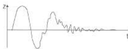
Figure 6. Graphical behavior of displacement vs time in an impact machine on the foundation system.
