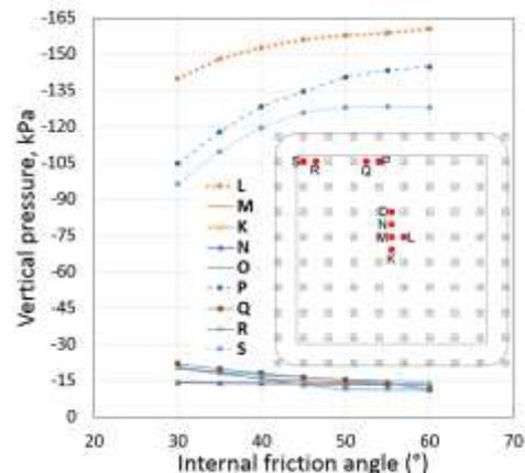
Figure 3. Numerical pressures on the soil and on pile caps
