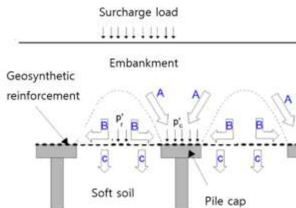
Figura 1. Load transfer mechanism in a piled embankment (Van Eekelen 2008)
