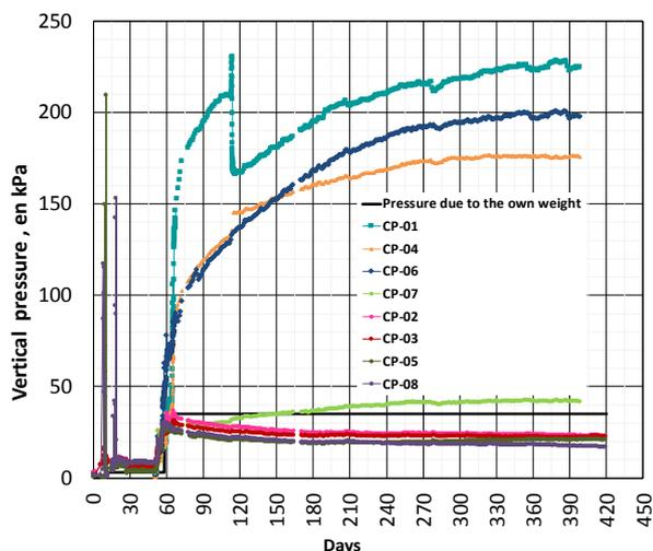
Figure 5. Measurements of the total pressure below the embankment.
