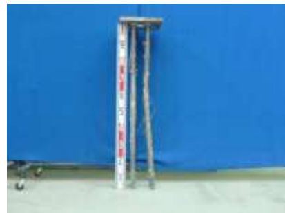
Figure 6. Pile deformation after the test in Case-1.
