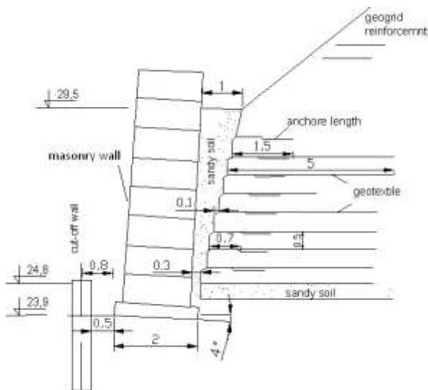
Figure 2. Cross section of retaining wall (Miszowska et al. 2015).
