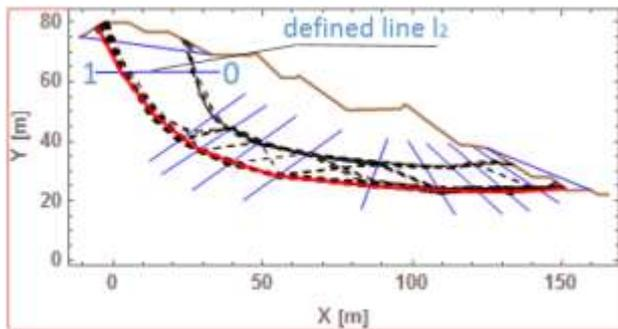
Figure 5. Definition of searching lines and last population of slip surfaces.
