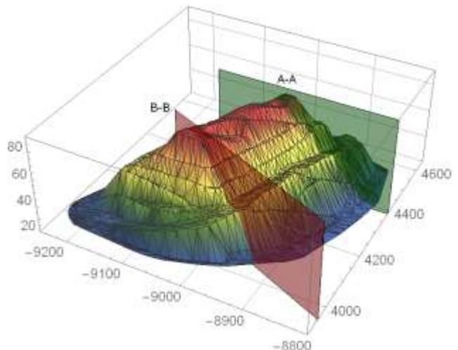
Figure 3. 3D visualization of Radiowo sanitary landfill and A-A cross-section.
