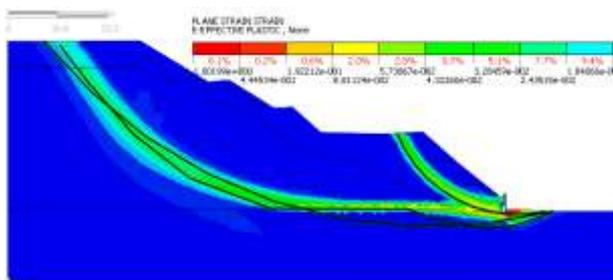
Figure 9. Slope stability analyses for reinforced slope using finite element method (cross section B-B).
