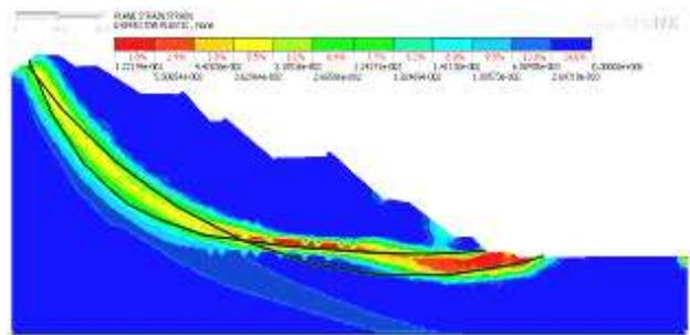
Figure 7. FEM results of accumulated plastic strain (Midas GTS NX) and LEM critical slip surfaces (D-Geo Stability).
