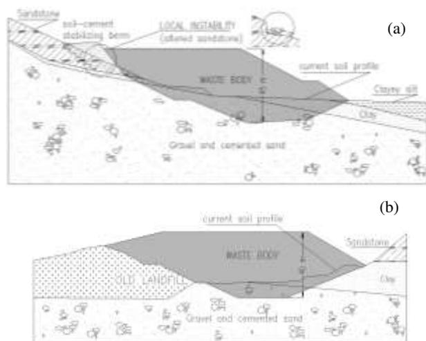
Figure 2. Cross sectional views of the landfill along the NW-SE direction –section 5 (a) and NE-SW direction –section C (b).
