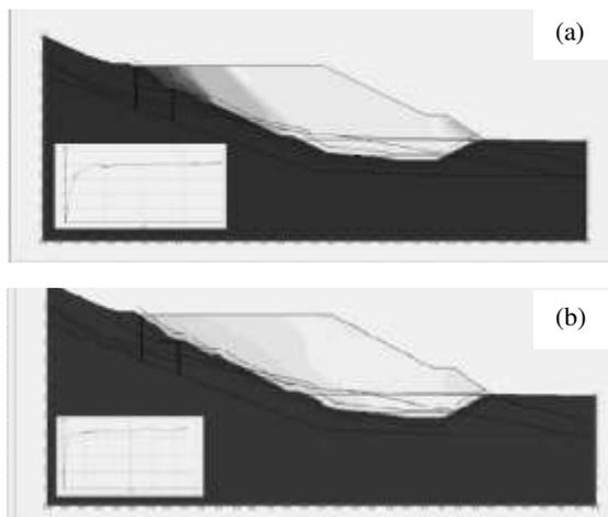
Figure 5. PLAXIS output of the *phi/c reduction* method under seismic conditions for section 5: (a) downward vertical inertial forces; (b) upward vertical inertial forces.
