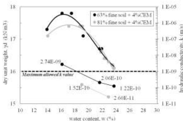
Figure 3. Compaction curves of soil A and B treated with 4% Portland cement (left axis) and hydraulic conductivity of the compacted specimens as a function of water content (right axis). Permeability tests were performed under an average effective stress of 25 kPa.
