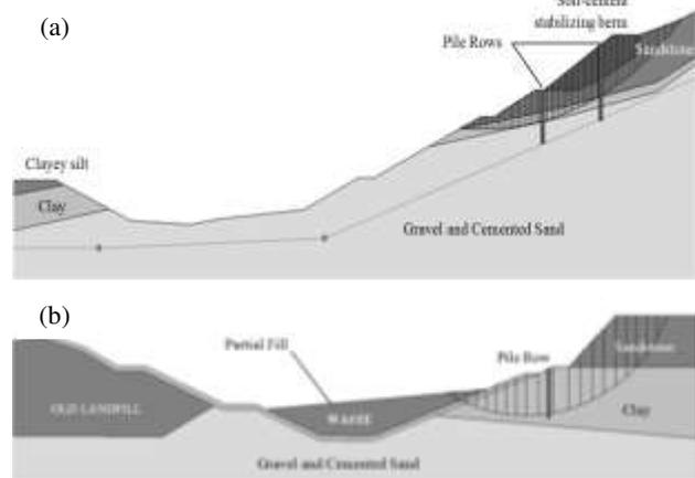
Figure 4. Critical slip surfaces in seismic conditions (a) along the NW-SE direction (STAP11); (b) along the NE-SW direction (STAP11)
