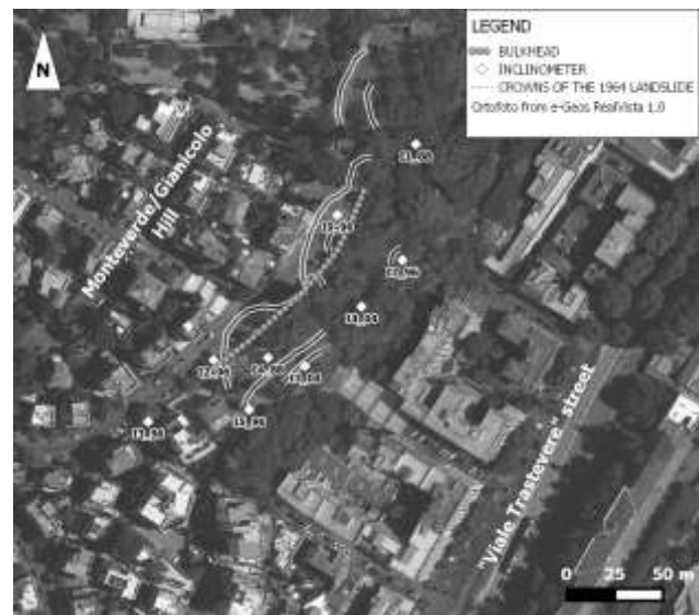
Figure 3. Location of monitoring network along Monteverde/Gianicolo Hill landslide.
