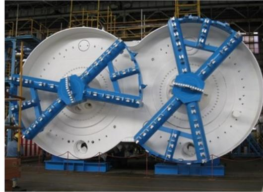
Figure 5. Double-O-Tube shield machine and concrete linings (from Moh and Hwang)
