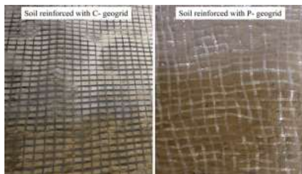
Figure 4. View of soil reinforced with C-geogrid and P-geogrid
