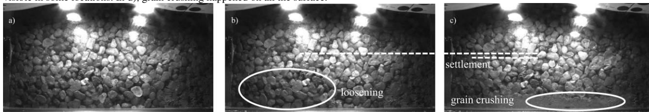
Figure 9. Image analysis with a Perspex container. a) initial configuration. b) during middle term cyclic shearing. c) End of cyclic test.
