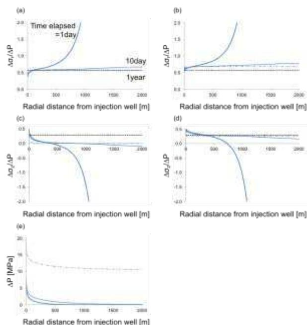
Figure 3. Spatio-temporal evolution of stress/pore-pressure change ratios when the hydraulic boundary of injection layer is closed. (a)  $\Delta\sigma_r/\Delta P$  at *middle*, (b)  $\Delta\sigma_r/\Delta P$  at *interface*, (c)  $\Delta\sigma_h/\Delta P$  at *middle*, (d)  $\Delta\sigma_h/\Delta P$  at *interface*, and (e)  $\Delta P$  in the injection layer.
