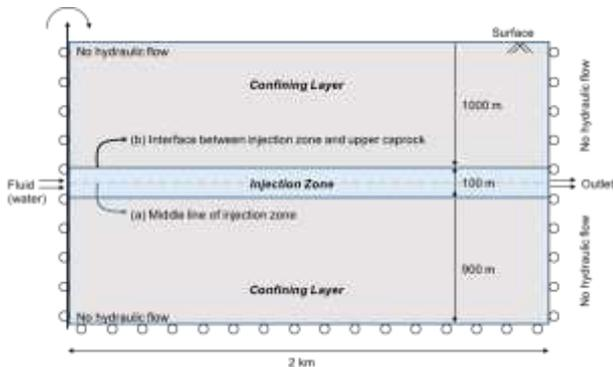
Figure 1. Simulation model for numerical experiments in this study: Geometry and the lines of interest (center line of injection layer and interface between injection layer and upper caprock).
