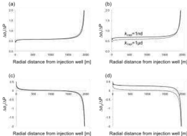
Figure 4. Spatial evolution of stress/pore-pressure change ratios with different caprock permeability  $k_{cap}$ . (a)  $\Delta\sigma_r/\Delta P$  at middle, (b)  $\Delta\sigma_r/\Delta P$  at interface, (c)  $\Delta\sigma_z/\Delta P$  at middle, and (d)  $\Delta\sigma_z/\Delta P$  at interface. Note: solid line represents when  $k_{cap}=1$  nd, and dashed line represents when  $k_{cap}=1$   $\mu$ d.
