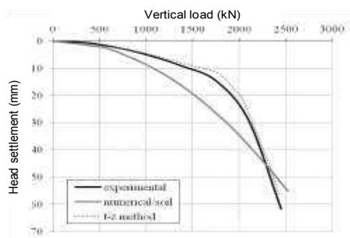
Figure 2. Pile head settlement (experimental=black line, numerical=grey line, t-z method=dotted grey line).
