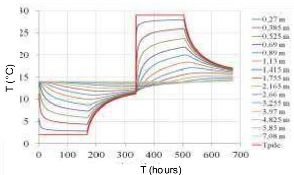
Figure 3. Pile temperature variation during a thermal cycle.
