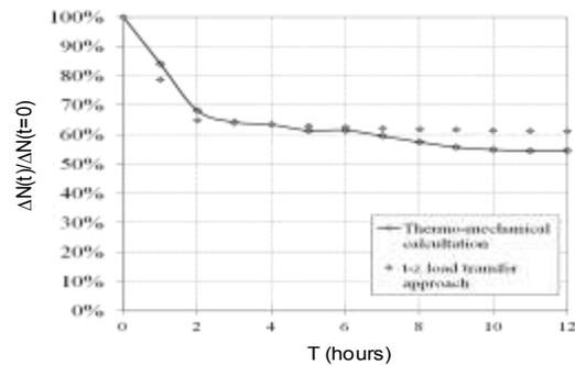
Figure 8. Ratio of the normal force variation at time t to that at t=0 during the cooling phase for the thermo-mechanical calculation (black), and t-z method (grey).
