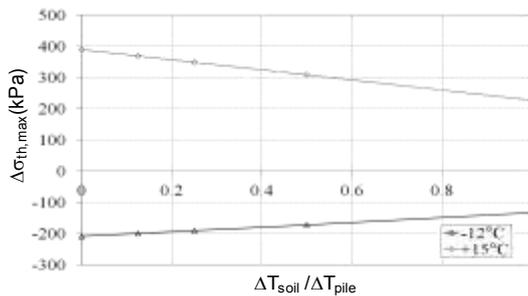
Figure 7. Variation of the maximum thermal normal stress with temperature.
