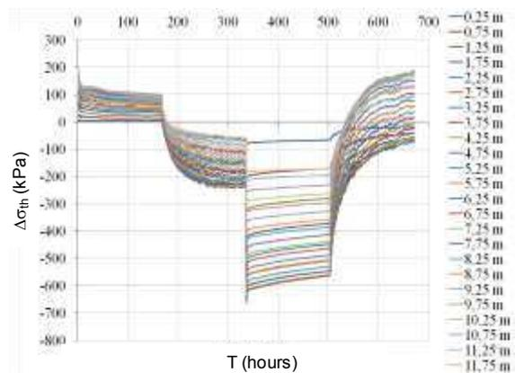
Figure 5. Variation of the thermally induced normal stress with time.
