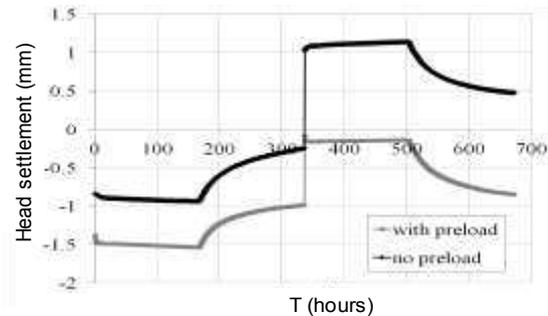
Figure 4. Variation of the thermally induced pile head displacement.
