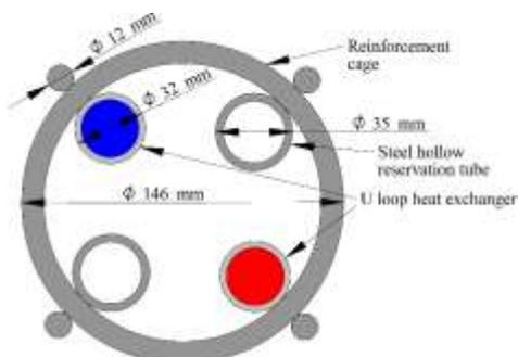
Figure 2. Schematic top view of the reinforcement cage.
