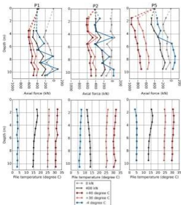
Figure 5. (top) Axial forces (negative sign = compression) and (bottom) temperatures in function of depth for energy piles P1, P2 and P5 at different loading steps. The legend refers to the temperatures at the inlet of the pile heat exchangers.
