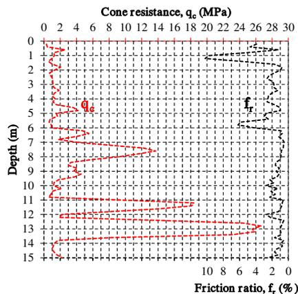
Figure 1. Typical CPT profile at the test site.
