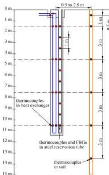
Figure 3. Cross-section of the pile and soil instrumentation.
