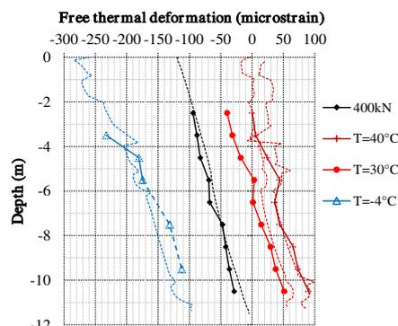
Figure 8. Comparison of the free thermo-mechanical deformation (negative sign is contraction) of the pile P1 as measured (solid lines) and as simulated by Plaxis (dashed lines).
