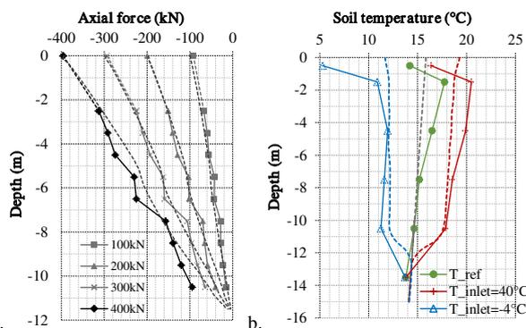
Figure 7. Comparison between the in situ measurements (solid line) and the Plaxis simulations (dashed line). (a) Axial forces in function of the pile depth at different load steps of the static load test on P1 (negative sign is compression). (b) Soil temperature at 0.5 m from the pile centre.
