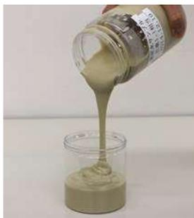
Figure 3. Heavy bentonite-based slurry.
