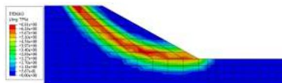
Figure 5. Contours of equivalent plastic strain using Abaqus.
