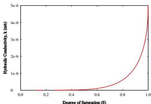
Figure 3. Permeability versus saturation
