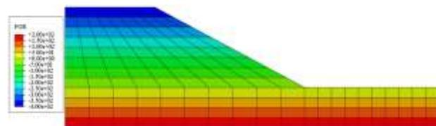
Figure 9. Pore water pressure distribution for Case III
