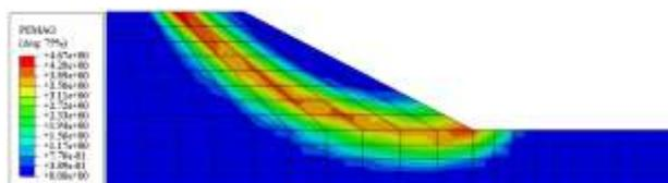
Figure 7. Contours of equivalent plastic strain for Case II
