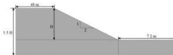
Figure 4. Geometry of a homogenous slope
