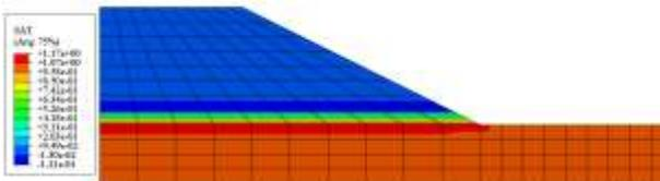
Figure 8. Degree of saturation for Case III
