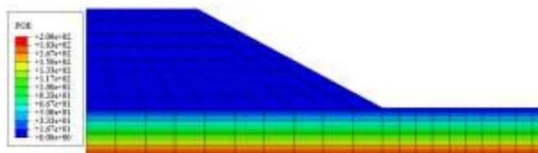
Figure 6. Pore water pressure distribution for Case II.
