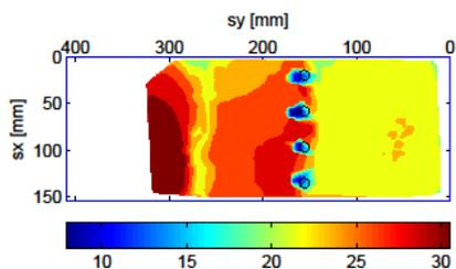
Figure 6. Surface displacement at 50g for test A4P. (Unit: mm)
