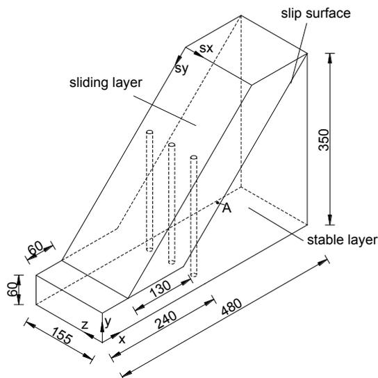
Figure 1. Geometry of the centrifuge model. (Unit: mm)
