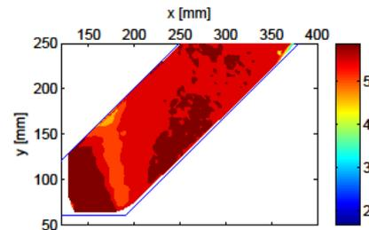
Figure 2. Soil displacement at 2.7g for test NP. (Unit: mm)
