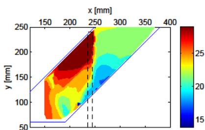
Figure 5. Total soil displacement at 50g for test A4P. (Unit: mm)
