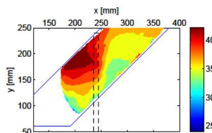
Figure 7. Total soil displacement at 45g for test A3P. (Unit: mm)
