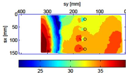
Figure 9. Surface displacement at 38g for test P4P. (Unit: mm)
