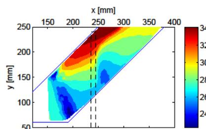
Figure 8. Total soil displacement at 38g for test P4P. (Unit: mm)
