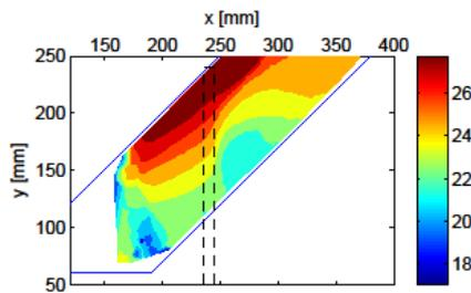
Figure 10. Total soil displacement at 30g for test P3P. (Unit: mm)
