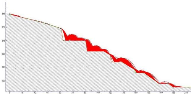
Picture N° 05: Rock block fall simulation for the natural slope.
