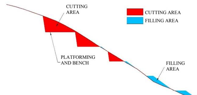
Picture N° 02: Natural slope's cut and fill.
