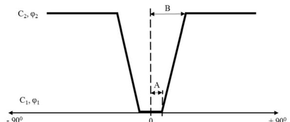
Figure 3. Scheme of parameters determining in the criterion of linear anisotropic strength (Snowden 2007).
