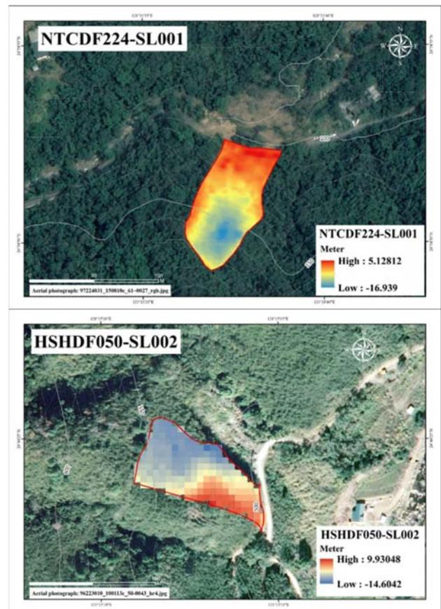
Figure 6. Illustration of topographic variations of two shallow landslides in Nantou County (upper) and Hsinchu County (lower). (Lin & Wang, 2018)
