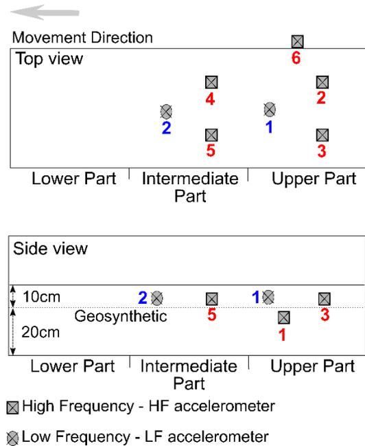
Figure 6 Accelerometers positions during the second experiment.
