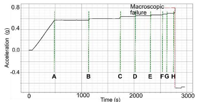
Figure 9 Acceleration measured with HFA-2 during the second experiment, in the axis parallel to the movement. Letters A to H correspond to the end of tilting events, showed in Table 3.
