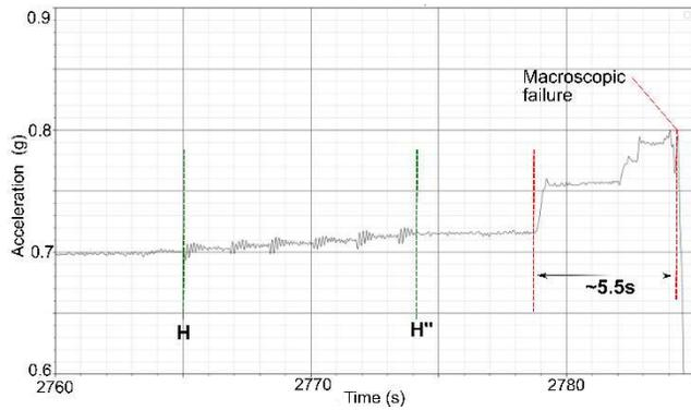
Figure 10 Detail of acceleration measured with HFA-2 in the axis parallel to the movement, close to macroscopic failure moment. Letters H' and H'' correspond to the beginning and the end of the 41° tilting event. Note the change in acceleration absolute value and pattern
