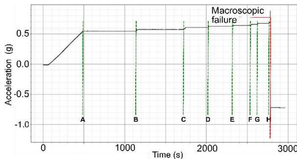
Figure 11 Acceleration measured with HFA-3 during the second experiment, in the axis parallel to the movement. Letters A to H correspond to the end of the tilting events showed in Table 3.
