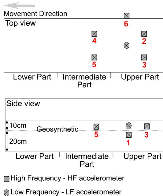
Figure 5 Accelerometers positions during the first experiment.
