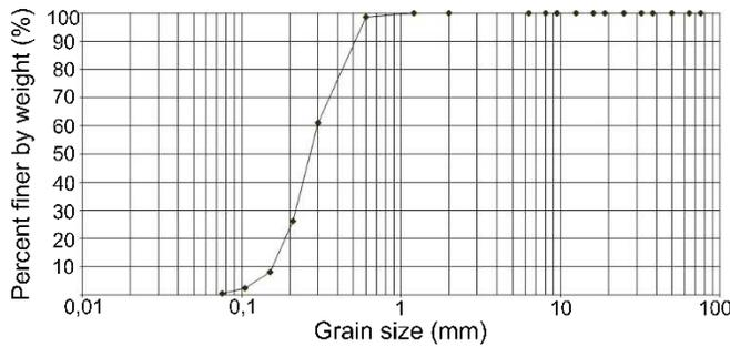
Figure 2 Grain-size distribution of the tested soil.
