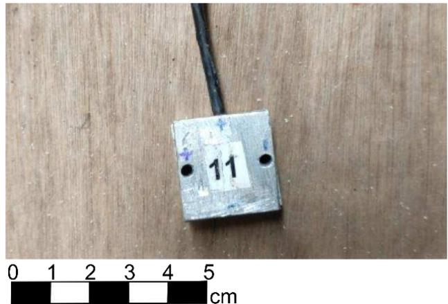
Figure 3 High frequency accelerometer (HFA).
