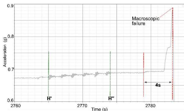
Figure 12 Detail of acceleration measured with HFA-3 in the axis parallel to the movement, close to macroscopic failure moment. Letters H' and H'' correspond to the beginning and the end of the 41° tilting event. Note the change in acceleration absolute value and pattern.
