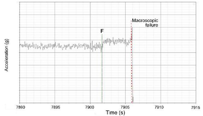
Figure 8 Detail of acceleration measured with HFA-3 in the axis parallel to the movement, close to macroscopic failure moment. Letter F corresponds to the end of the tilting 41° event, before the macroscopic failure.
