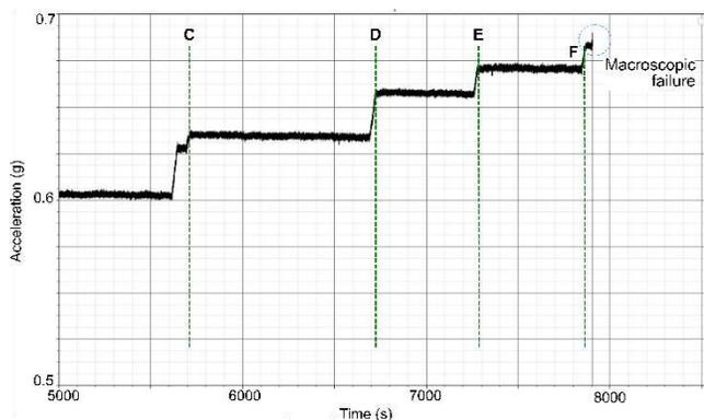
Figure 7 Acceleration measured with HFA-3 during the first experiment. Letters C to F with green lines correspond to the end of tilting events, showed in Table 2.
