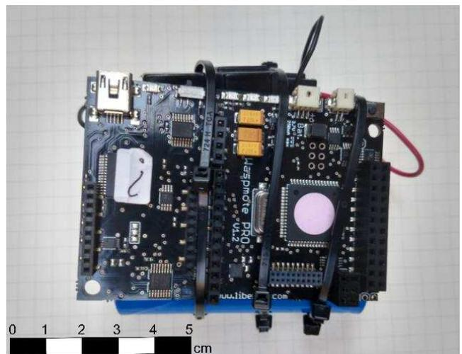
Figure 4 Low frequency accelerometer (LFA).
