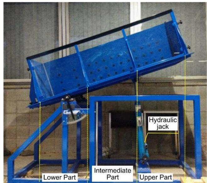
Figure 1 Tilting flume developed for the research.
