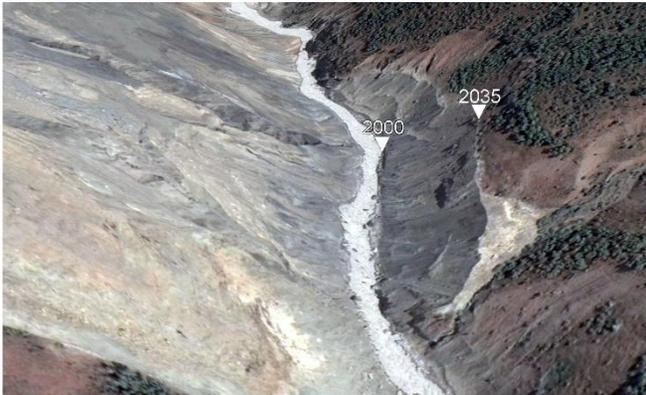
Figure 3. Remnant of the completely eroded dam in the Ragnow River valley. 3D Google Earth image.
