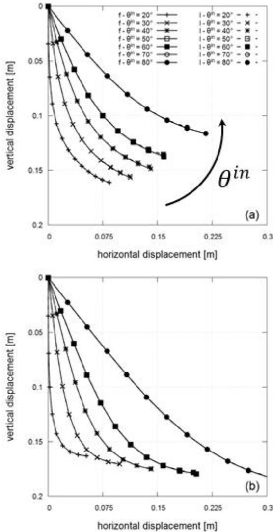
Figure 6 Block trajectories for blocks with free and locked rotating: (a) spherical blocks, (b) prismatic with triangular base blocks.
