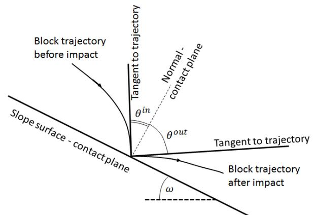
Figure 1. Slope angle  $\omega$ , block trajectory before and after the impact, normal direction to the contact plane, incident and restitution angles  $\theta^{in}$  and  $\theta^{out}$ , respectively.
