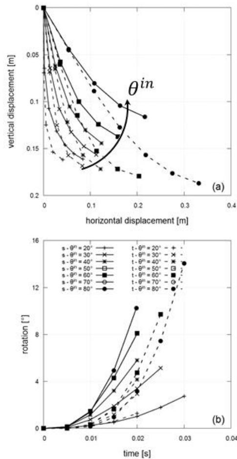
Figure 5 Numerical simulation results obtained considering a slope inclined of  $20^\circ$  and spherical and triangular blocks impacting with different inclinations. (a) Blocks trajectories during sinking in the layer; (b) rotation versus time. The prefixes "s-" and "t-" stand for sphere and triangular prisms, respectively.
