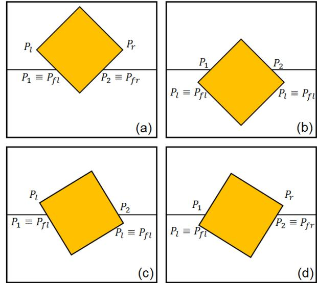
Figure 2. Position of the  $P_1$ ,  $P_2$ ,  $P_l$ ,  $P_r$ ,  $P_{fl}$  and  $P_{fr}$ . (a) low level of penetration; (b) high level of penetration; (c) middle level of penetration with a block rotated clockwise; (d) middle level of penetration with a block rotated anticlockwise.
