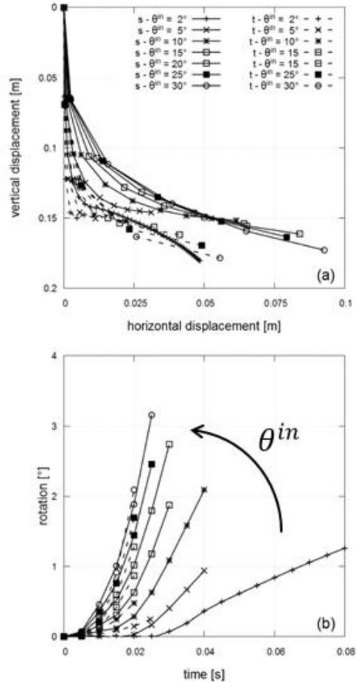
Figure 7 Vertical impacts for both spherical ("s-") and prismatic blocks with triangular base ("t-"): (a) blocks trajectories, (b) time evolution of blocks rotation.
