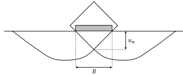
Figure 3. Visco-plastic mechanism occurring at the bottom part of the block. The mechanism is equivalent to failure mechanism generated in a shallow foundation.
