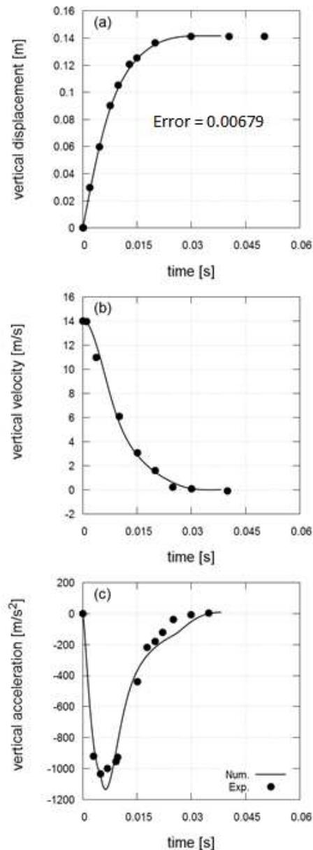
Figure 4 Comparisons between the advanced rheological model results and the experimental data from Labiouse et al. (1994). Evolution with time of (a) vertical displacement; (b) vertical velocity and (c) vertical acceleration.
