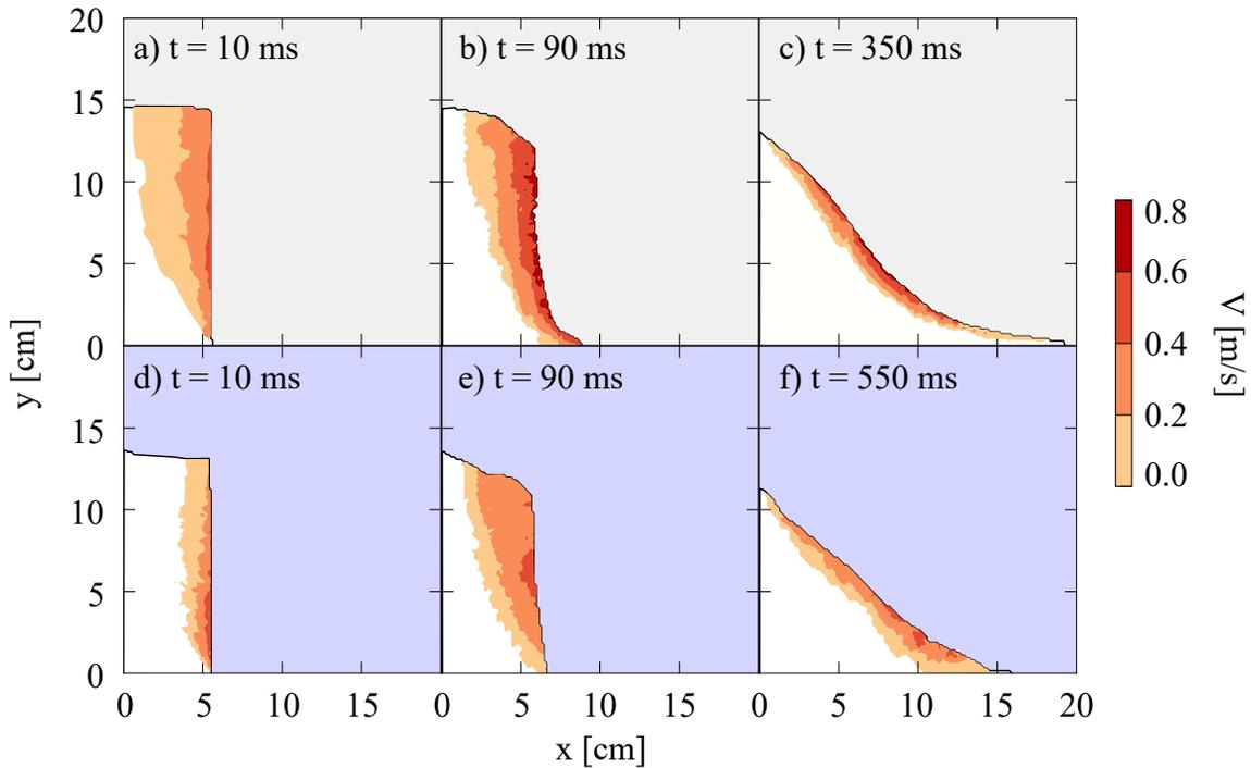
Figure 2: Velocity fields for a dry collapse (a-c) and a submerged collapse (d-f) at different instants of collapse. The last frame in each scenario (c & f) corresponds to the instant when the granular mass reaches its final runout ( $L_f$ ) while maintaining a shallow layer of particles moving on its surface.
