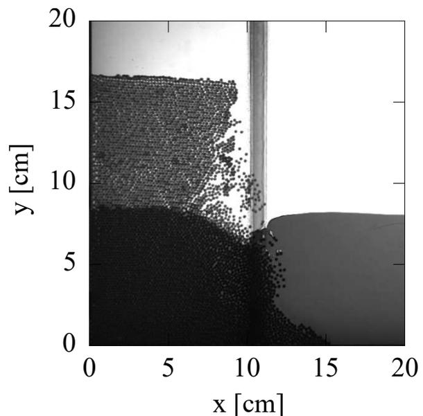
(b) Column collapse at  $t = 230$  ms under partially-saturated conditions
