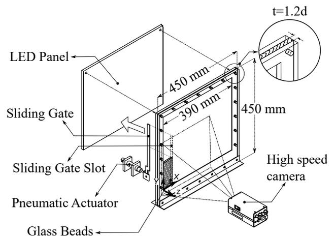
Figure 1: Planar granular column collapse setup.
