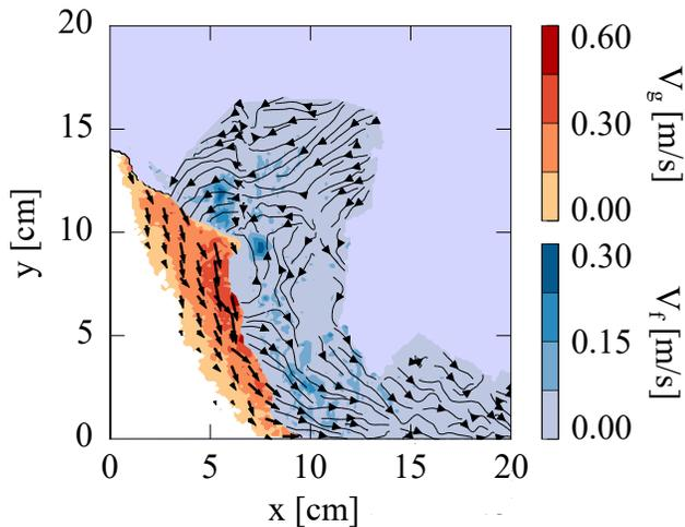
Figure 3: Velocity fields of a submerged collapse over the granular mass and the surrounding fluid. The fluid motion is captured by applying a liquid dye (Pinzón and Cabrera, 2019).
