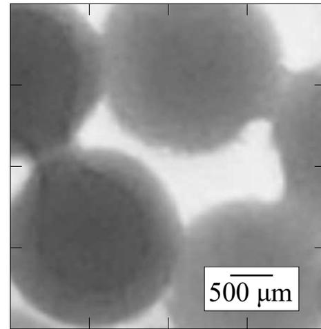
(a) Close-up to the menisci between beads after the column desaturation and prior to collapse.
