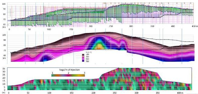
Figure 11 - Shear wave velocity profile through the central part of the project.
