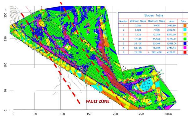
Figure 2 – Slopes map of the project area showing the fault zone.
