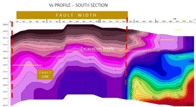
Figure 10 - Shear wave velocity profile through the central part of the project.
