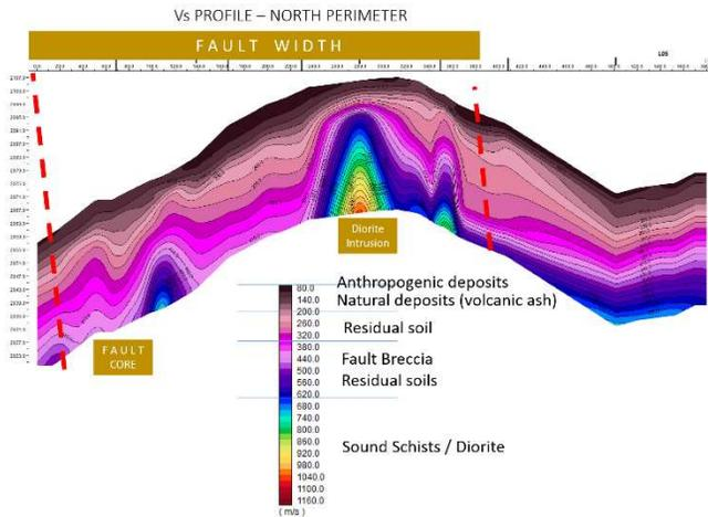
Figure 9 – Shear wave velocity profile along the project's north perimeter.
