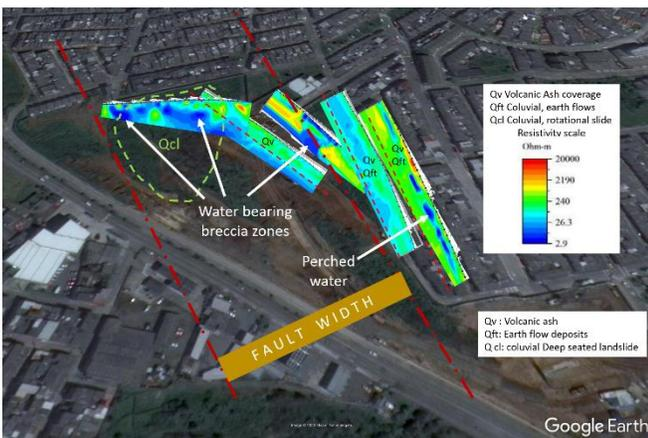
Figure 3 – Resistivity tomography sections.
