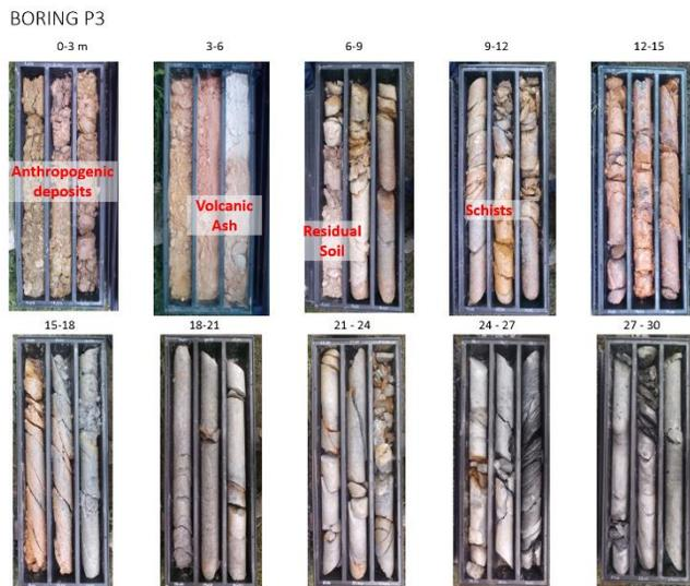
Figure 5 - Photographic record of P3 drilling located the fault zone in the central part of the project.
