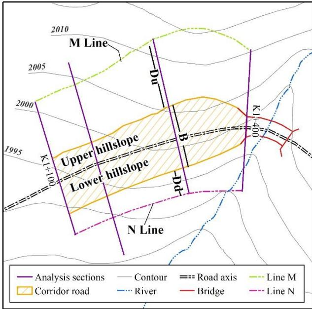
Figure 2. Definition of the hillside analysis area up and down the corridor.
