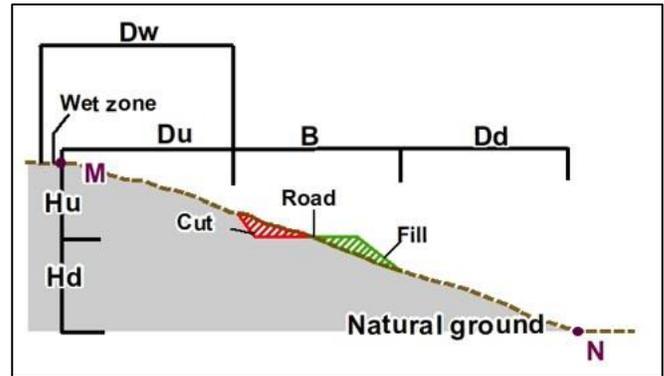
Figure 1. Definition of analysis sections for hillside characterization.
