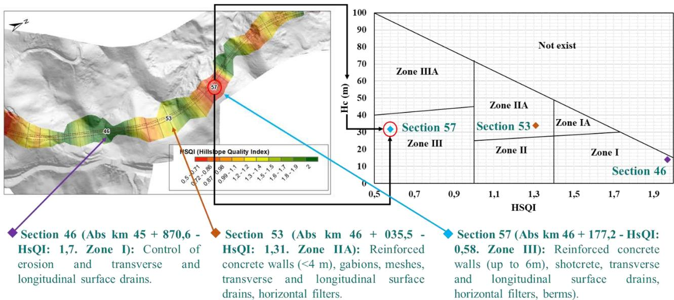
Figure 10. Zoning and performance graph for three particular analysis sections.
