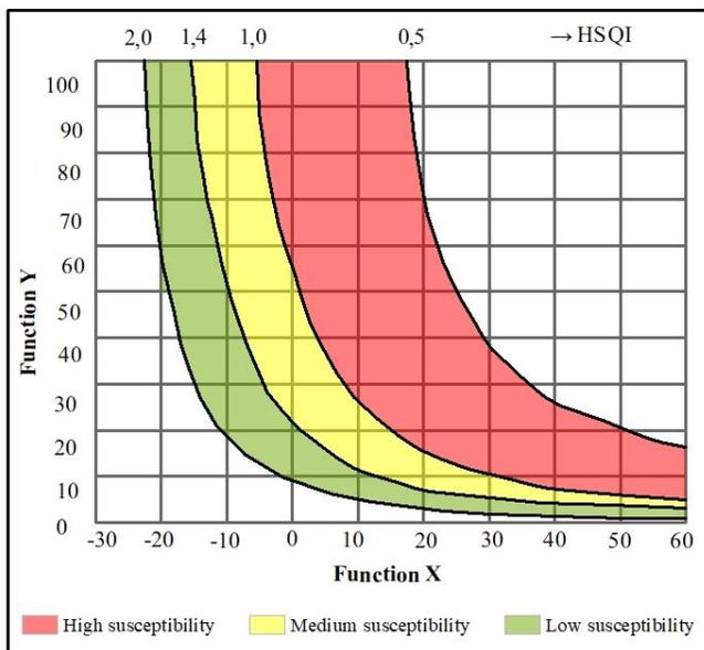
Figure 3. HsQI for landslides with rupture mechanisms not structurally controlled (circular failure).
