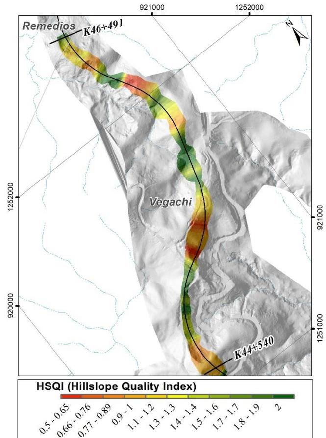
Figure 8. Zoning of susceptibility to landslides of the road corridor.
