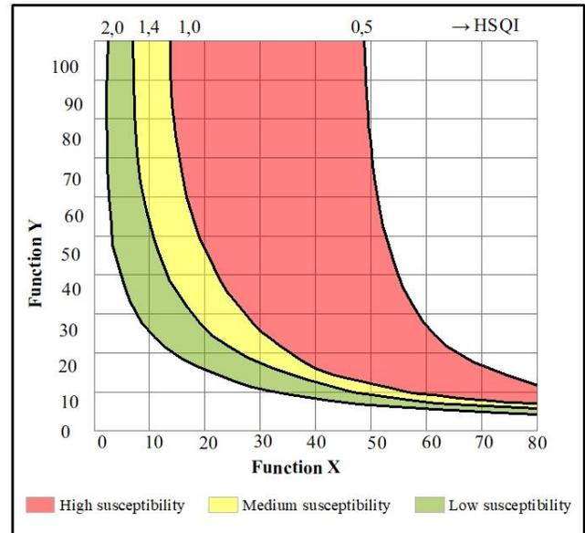
Figure 4. HsQI for landslides with structurally controlled rupture mechanisms (planar failure).
