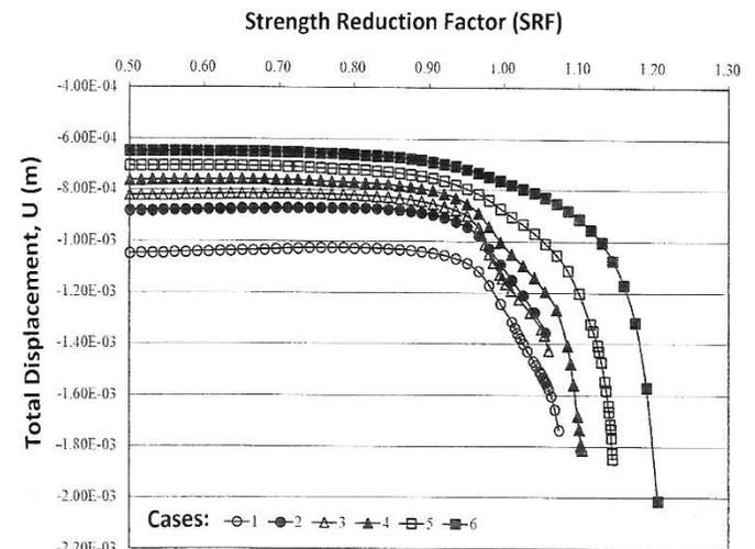
Figure 6. Relationship between the total displacement U and the strength reduction factor (SRF) used to obtain the FOS.
