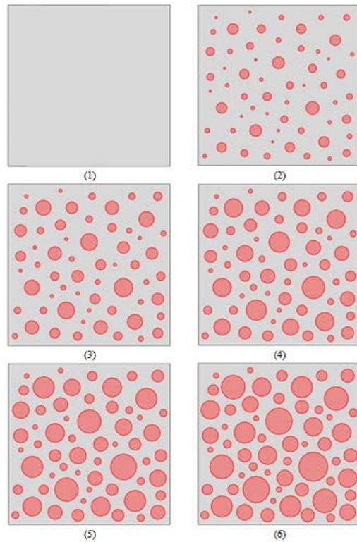
Figure 3. Slope with six different concentrations by volume,  $C$ , of the large dispersed rock pieces that were assumed to be welded to the soil matrix and were randomly distributed according to their sizes.
