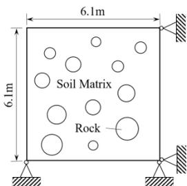
Figure 2. Slope used for the finite element analysis
