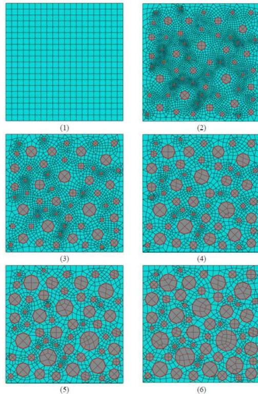
Figure 4. Mesh plan for the vertical slope and the six cases with different volumen concentration,  $C$ , of rocks. The rocks were assumed to be welded to the soil matrix and were randomly distributed according to their sizes
