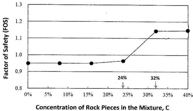
Figure 7. Relationship between the FOS and C for the six different cases shown in Fig. 3
