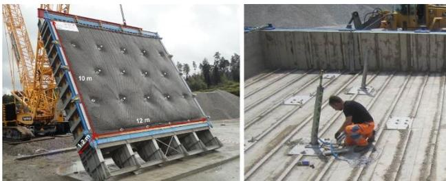
Figure 5. Test setup before the rupture of flexible facing and frame sizes and box frame empty
