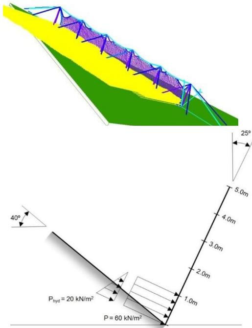
Figure 18. First load case for rockfall barrier dynamic impact pressure of 60 kN/m<sup>2</sup> acting over flow height of 1 m.
