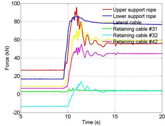
Figure 6. Load combination during impact (dynamic and static), influence into ropes.
