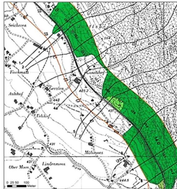
Figure 17. High intensity rockfalls, for a 100 year return period, at Balisberg area.
