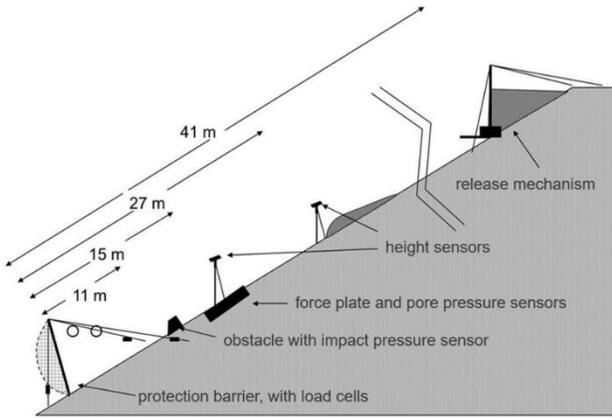
Figure 3. Experiment setup. Test channel in the cement quarry, Veltheim (Switzerland)
