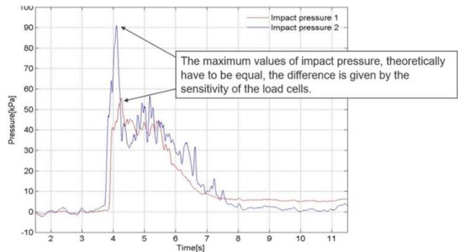
Figure 7. Impact pressure measurement at the test site.
