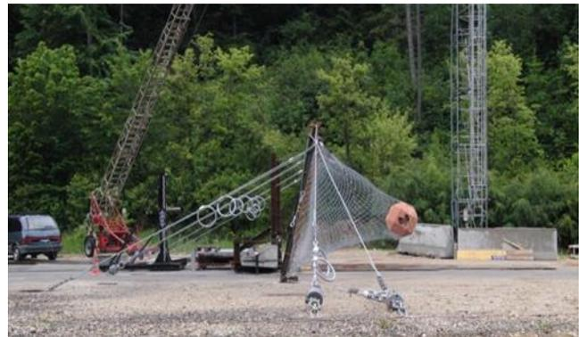
Figure 15. EOTA standard block 1600 kg, with 500 kJ energy impact into a standard SL-150 shallow landslide barrier.
