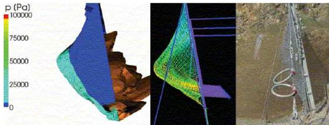
Figure 4. Modelled shallow slide impact on the flexible barrier with coupled OPEN FOARM software (fluid code) and modelled with FARGO software (Finite Element Software for barrier design).
