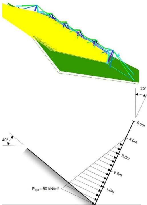
Figure 19. Second load case of hydrostatic pressure acting over filling height of 4 m.
