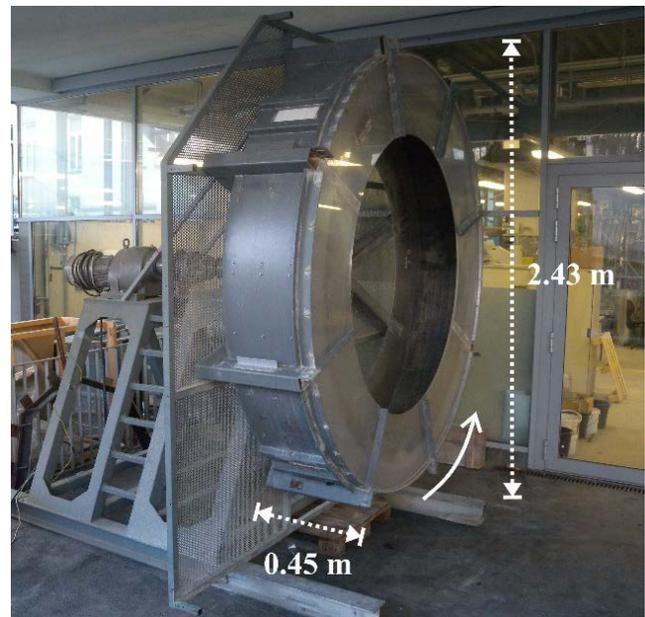
Figure 4. Rotating drum setup at IAN-BOKU, Vienna.
