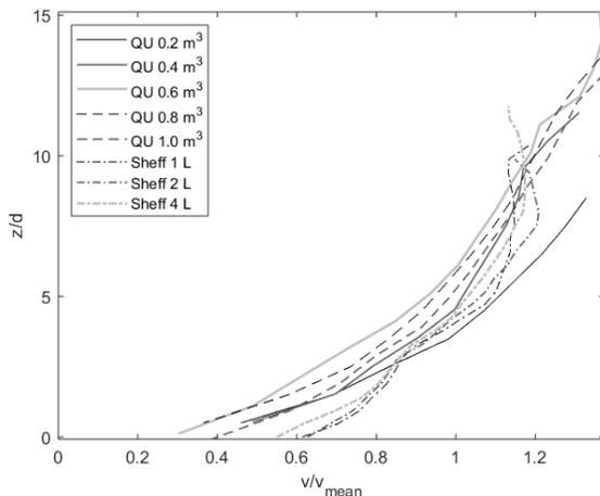
Figure 5. Dry flows of 3mm ceramic particles for flume tests. Downstream velocity profile at sidewall normalized by mean flow velocity against flow height normalized by particle size.
