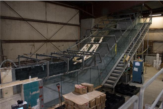
Figure 2. Large scale flume at Queen's University, Kingston.
