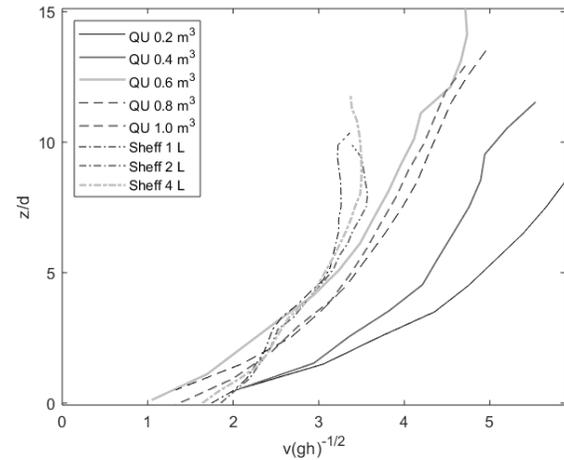
Figure 6. Dry flows of 3mm ceramic particles for flume tests. Downstream velocity profile at sidewall normalized by  $\sqrt{(gh)}$  against flow height normalized by particle size.
