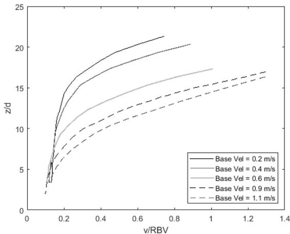
Figure 7. Dry flows of 3 mm ceramic particles for drum experiments. Velocity profiles for 49kg normalized by rotational base velocity.
