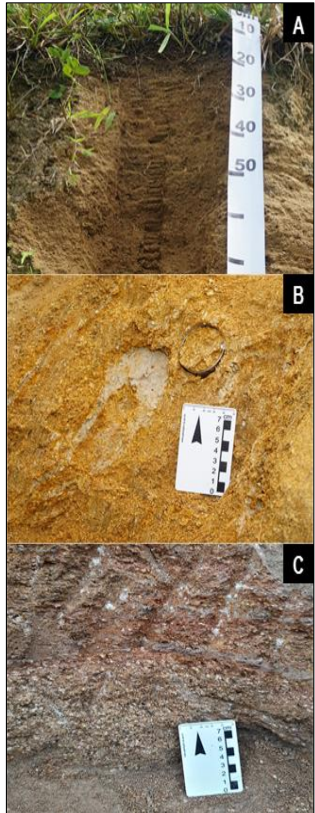
Figure 4: Weathering Profile: (A) Residual Soil; (B) Saprolite II; (C) Saprolite I.
