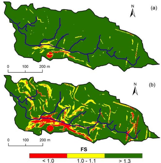
Figure 4. Factor of safety (FS) using TRIGRS: (a) before rainfall (dry conditions); (b) groundwater level at the soil surface (saturated conditions).
