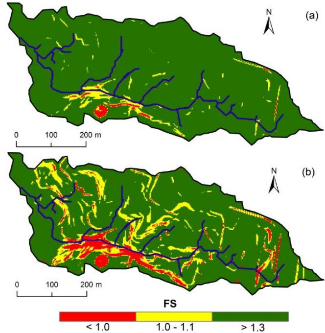
Figure 3. Factor of safety (FS) using Papa et al. (2013) model: (a) before rainfall (dry conditions); (b) groundwater level at the soil surface (saturated conditions).
