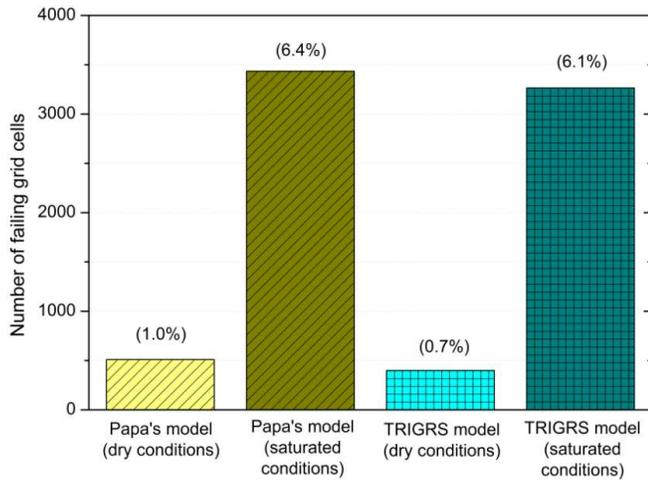
Figure 5. Number of grid cells and failure area for the dry and saturated scenarios, with Papa's and TRIGRS models.
