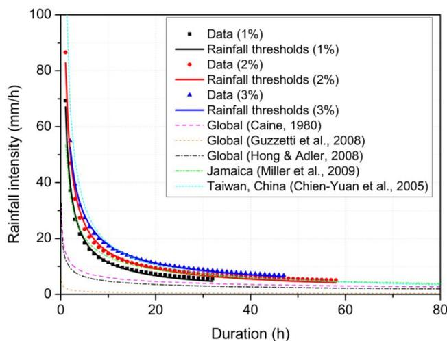
Figure 6. Rainfall thresholds using Papa et al. (2013) for different  $a_c$  values. The points (data) represent the critical I-D values calculated in the simulation.
