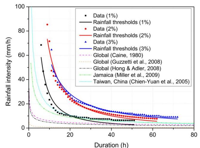
Figure 7. Rainfall thresholds using TRIGRS for different  $a_c$  values. The points (data) represent the critical I-D values calculated in the simulation.
