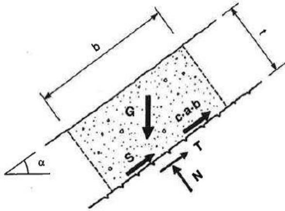
Figure 1. All forces acting on the body mass to determine the shear force S required for a certain safety (Rüegger & Flum, 2000) (1)
