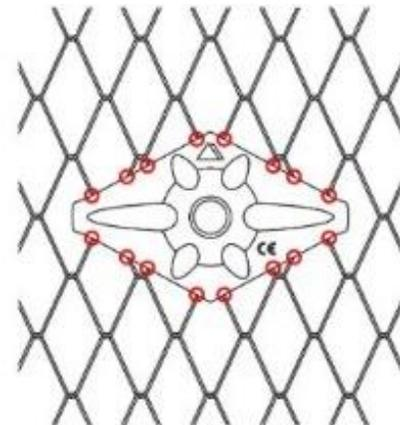
Figure 2 Contact points between the wire net and plate in direction perpendicular to the slope surface (Rüegger & Flum, 2000)
