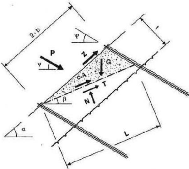
Figure 3 Forces actin on the wedge-shaped body (Rüegger & Flum, 2000)
