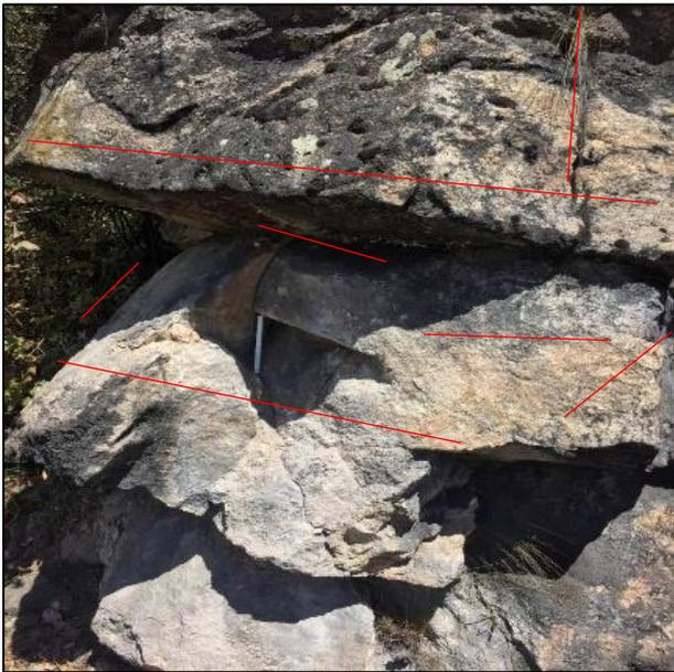
Figure 4 Incidence of crossing joints creating smaller blocks
