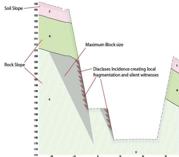
Figure 5 Rock slope profile showing the maximum block and the incidence of diaclases creating smaller blocks.
