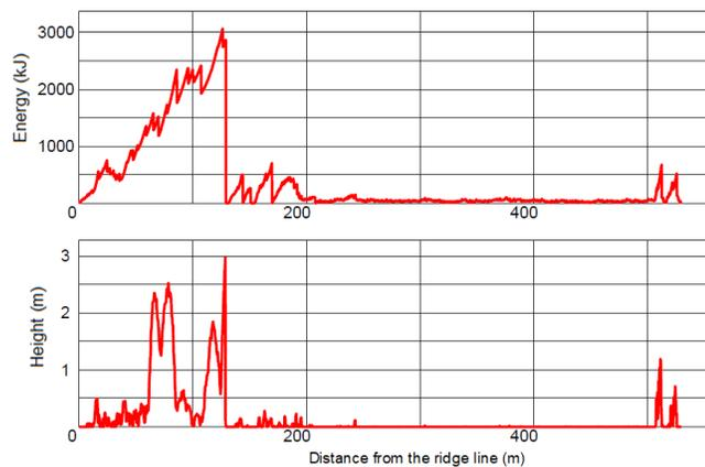
Figure 7. Results of the analyses to the section 3, using properties given by the Combination 3 (a – energy; b – bounce height).
