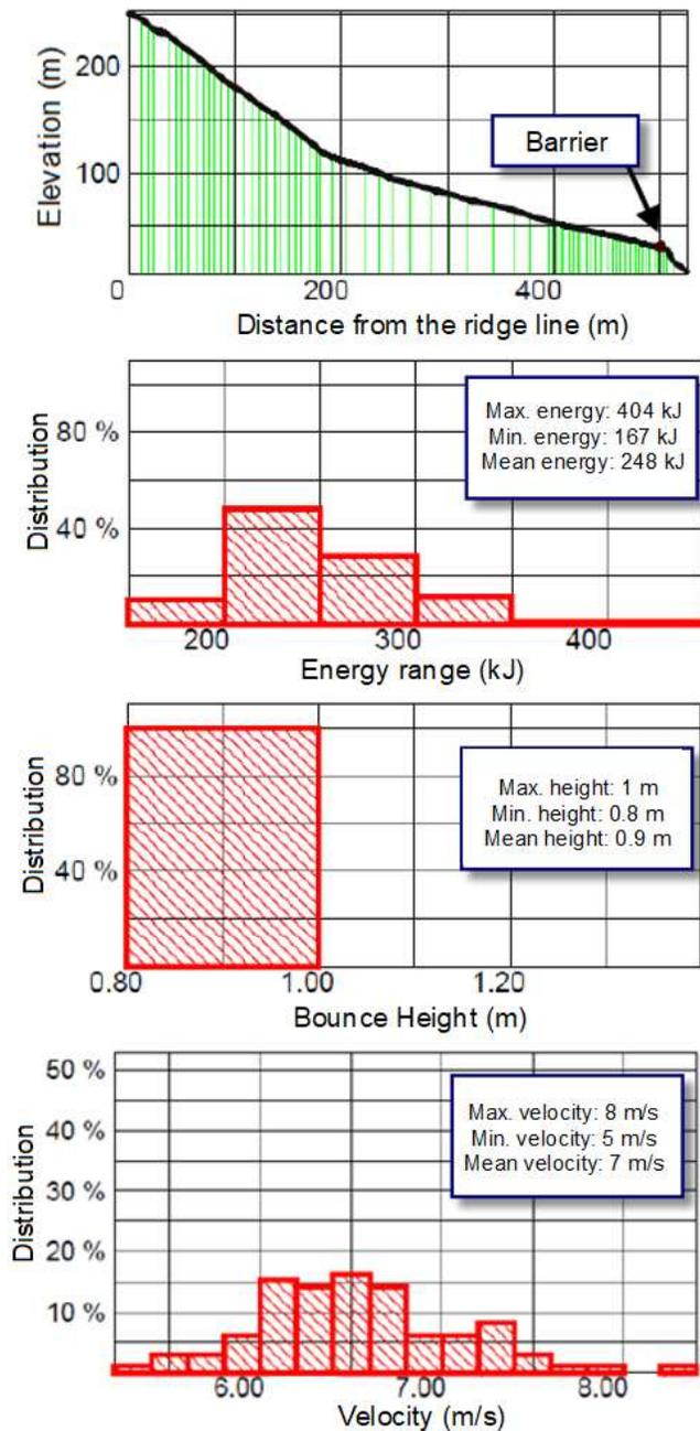
Figure 10. Results of the statistical analyses of energy, impact height and velocity for section 3.
