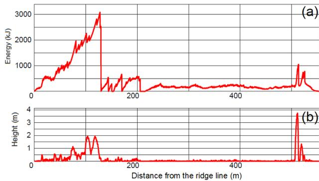
Figure 6. Results of the analyses to the section 3, using properties given by the Combination 1 (a – energy; b – bounce height).
