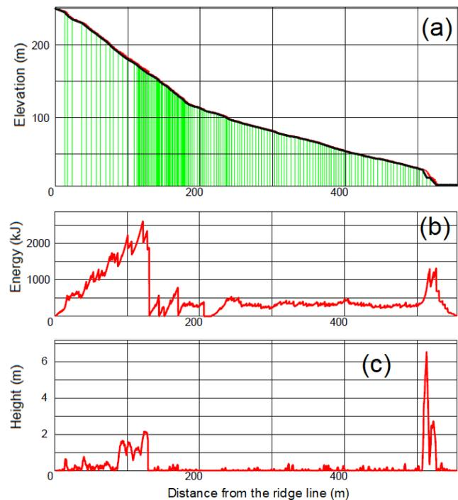
Figure 5. Results of the analyses to the section 3 (a - surface profile and rock path; b – energy; c – bounce height).
