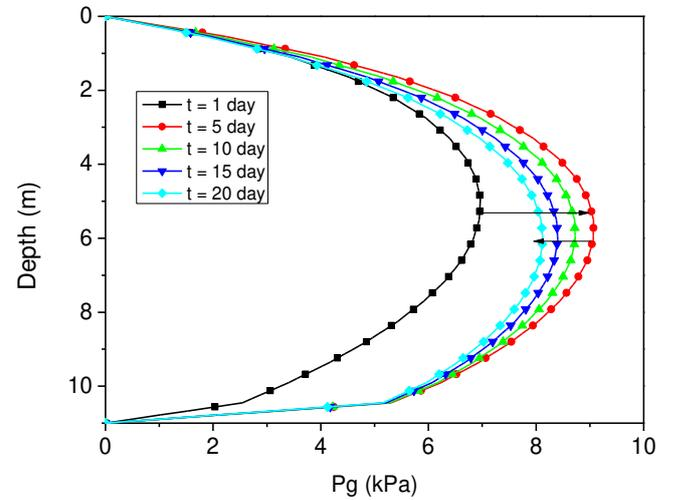
Fig. 5. Landfill gas pressure distribution.
