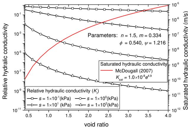
Fig. 3. The effect of void ratio on hydraulic conductivity.
