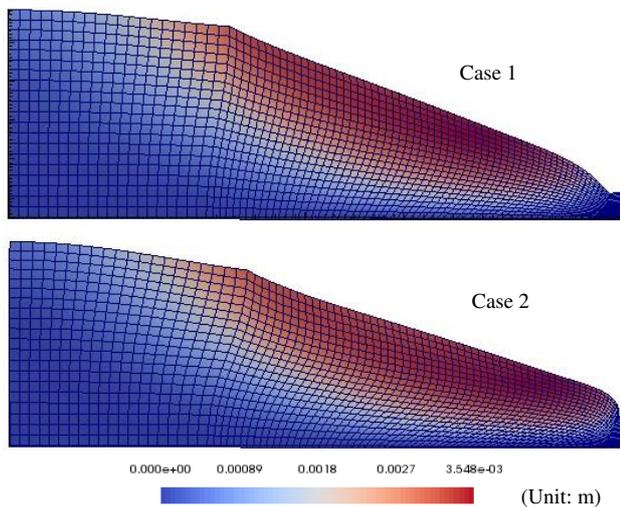
Fig. 7. The comparison of deformation results between case 1 (without considering the effect of coupled process) and case 2 (considering the effect of coupled process).
