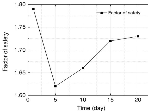
Fig. 6. The relationship between  $FS$  and biodegradation time.
