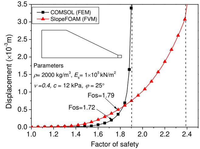
Fig. 1. The determination of factor of safety.
