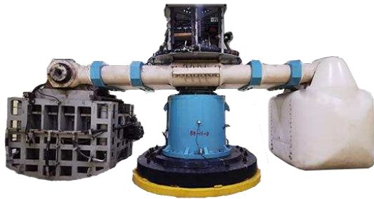
Fig. 1. Photo of the IWHR horizontal-vertical centrifuge shaker
