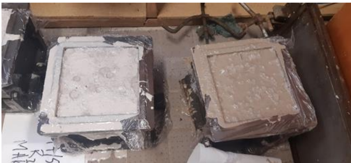
Figure 5: Moulds filled with the mixtures of binder with carbonate limestone and marble sludges and Recapoli resin.
